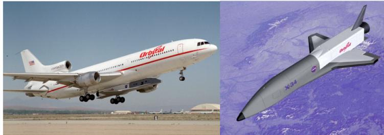
Figure 3.13: The X-34 vehicle underneath of the L-1011 carrier (left), free flight test (right) [2]
