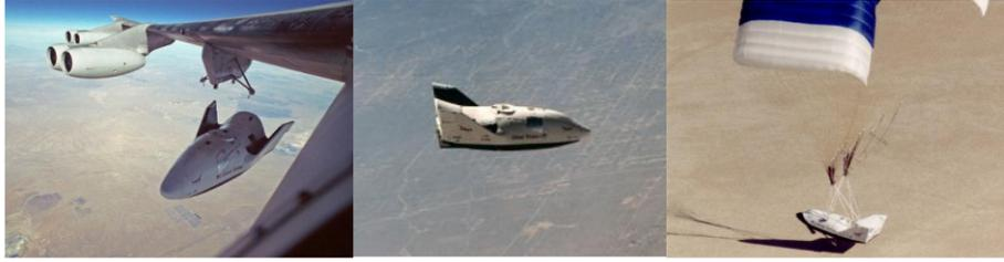
Figure 3.16: Drop test including parafoil landing of the X-38 vehicle [2]
