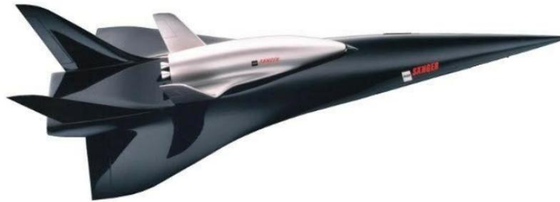
Figure 1.4: SANGER configuration with HORUS Orbiter
