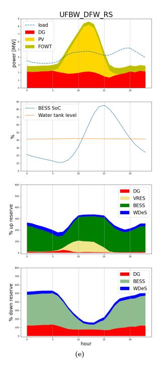
**Figure 5.6:** Yearly average of each hour of the day for: power and load curves (first row), BESS SoC and water tank level second row), up and down reserve in relation to the  $R_{rq}$  and  $Q_{rq}$  requirements (third and fourth rows, respectively), where light colors correspond to the unconstrained reserve in the scenario.
