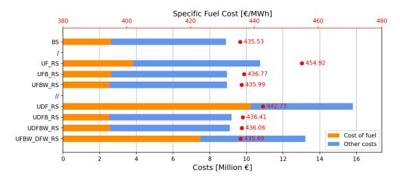
**Figure 5.1:** Objective function results and marginal costs of DGs (lower scale). Specif fuel consumption (upper scale)
