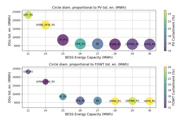
Figure 5.2: Scatter plot of PV vs FOWT curtailment. The x-axis represents BESS energy capacity, the y-axis shows the total energy supplied by DGs, the color map indicates the curtailment level, and the circle diameter is proportional to the total energy supplied.
