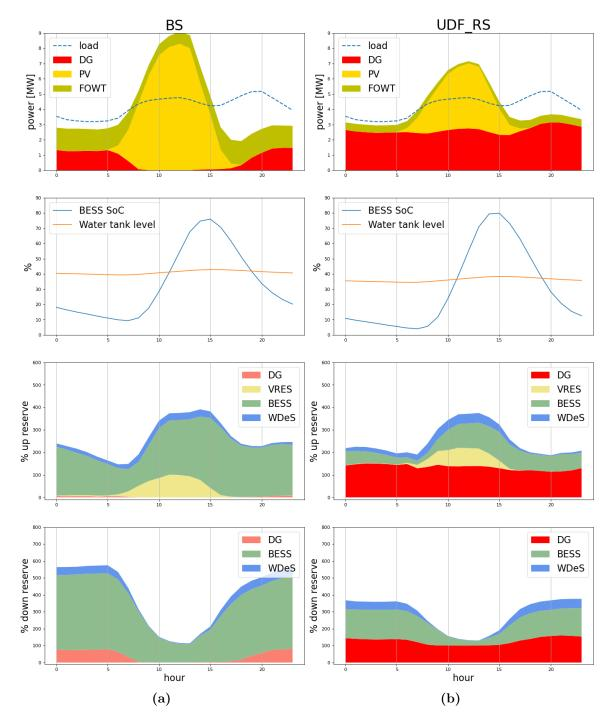
**Figure 5.6:** Yearly average of each hour of the day for: power and load curves (first row), BESS SoC and water tank level (second row), up and down reserve in relation to the  $R_{rq}$  and  $Q_{rq}$  requirements (third and fourth rows, respectively), where light colors correspond to the unconstrained reserve in the scenario.
