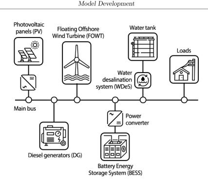
Figure 4.1: Model architecture. Images from Flaticon.com
