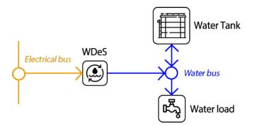
**Figure 4.2:** Model representation of WDeS, Tank and Water Load connected to the network. Images from Flaticon.com
