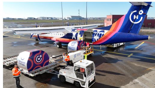
(b) Dash 8 retrofitted by Universal Hydrogen. Source: https://hydrogen.aero/
