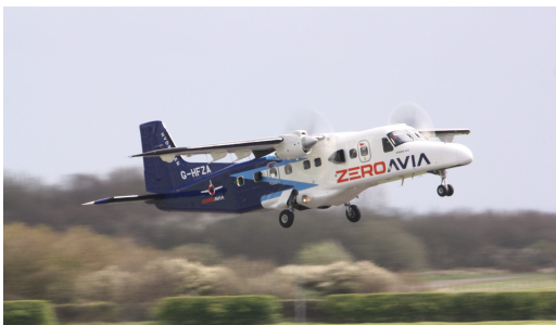
(a) Dornier 228 retrofitted by ZeroAvia. Source: https://zeroavia.com/
