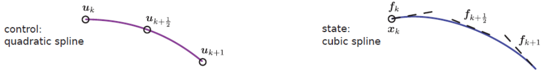
Figure 3.7: Quadratic and cubic spline segments adopted to approximate the control and state trajectories for Hermite–Simpson collocation.[13]
