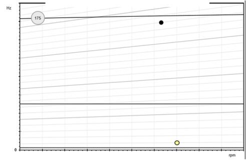
(b) Campbell Diagram with 30g/s exciting airflow and 5rpm/s deceleration
