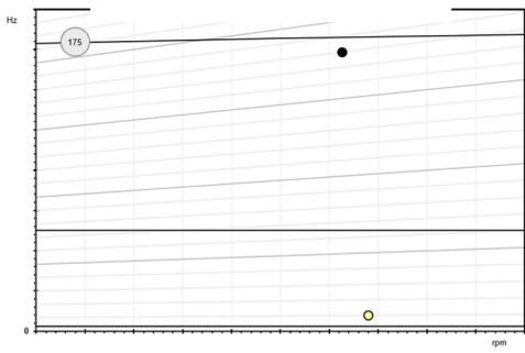
(a) Campbell Diagram with 30g/s exciting airflow and 5rpm/s acceleration
