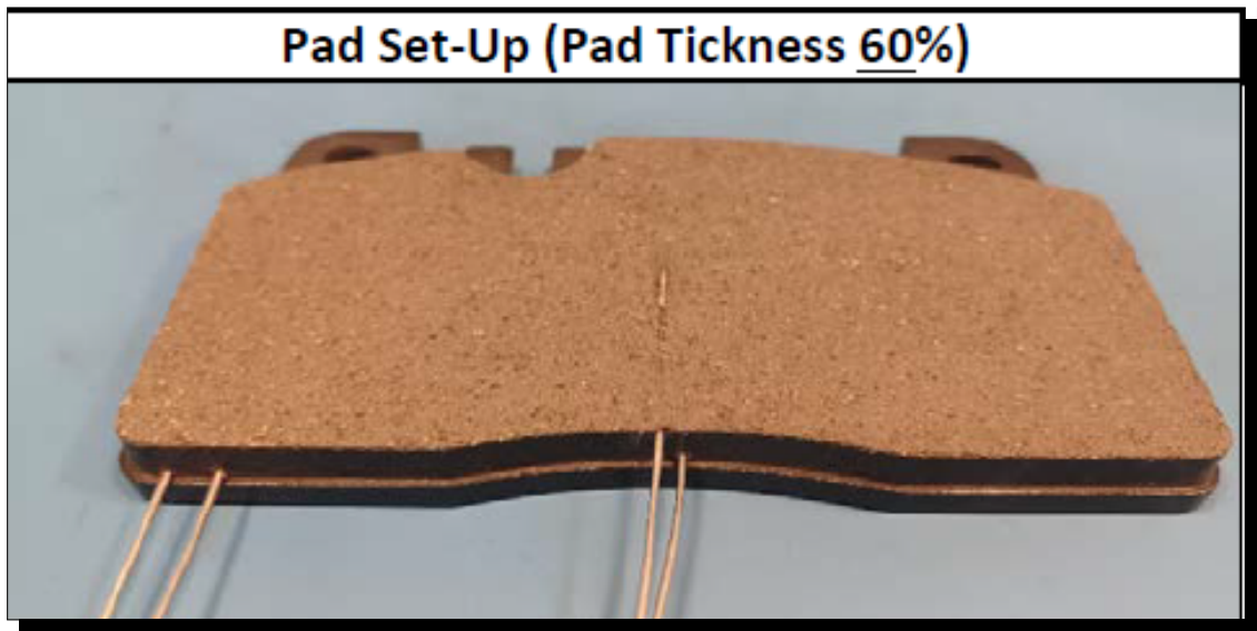
Figure 3.12: Real distribution of the sensors in the Pad used to collect data. The 2nd sensor position could not be the one expected
