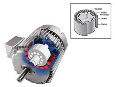
Figure3. PMSM Model Illustration, taken from [39]
