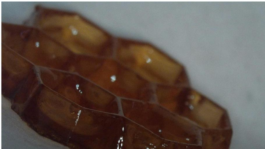
*Figure 52. Honeycomb printed using P3 resin.*
