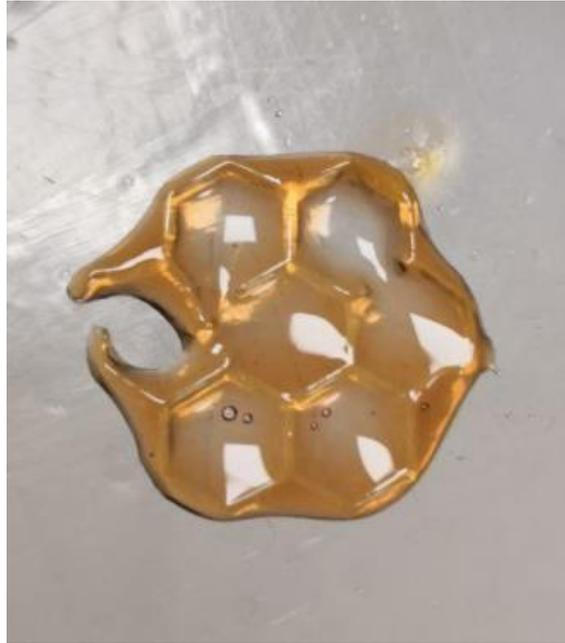
Figure 50. Result of a printed honeycomb using P1 resin with P3 printing parameters.
