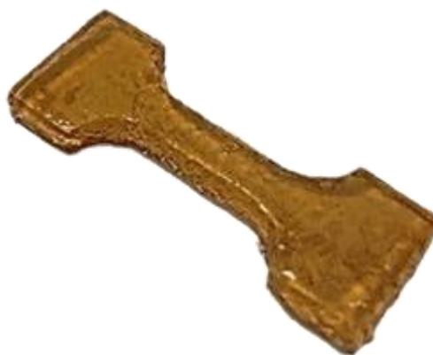
*Figure 41. Dogbone sample for tensile testing.*
