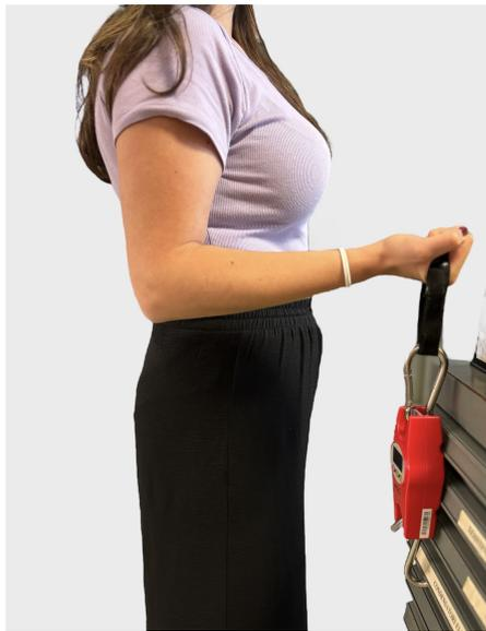
**Figure 6.1:** Estimation of Maximal Voluntary Contraction (MVC): this is the experimental set-up followed during the measure of the MVC of each subject.
