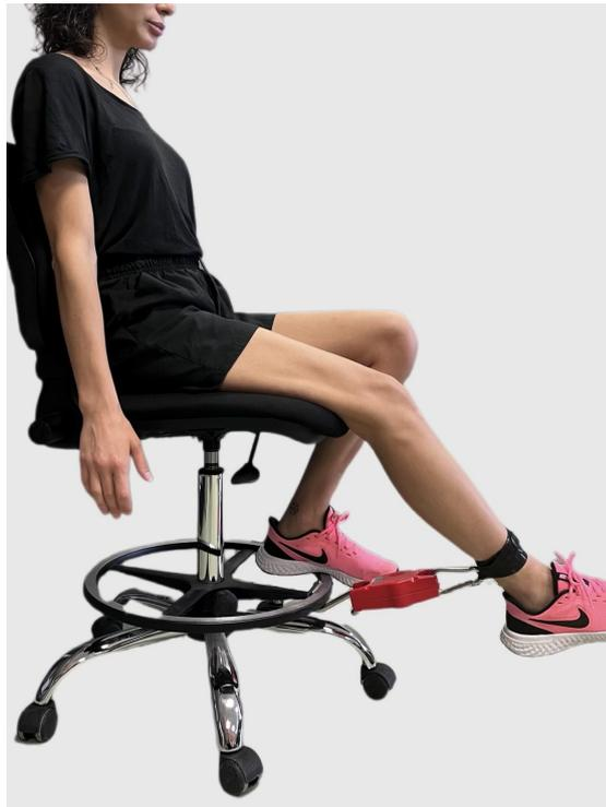
**Figure 8.3:** Estimation of Maximal Voluntary Contraction (MVC) of *quadriceps femoris* performing an *knee extension*: this is the experimental set-up followed during the measure of the MVC of each subject.
