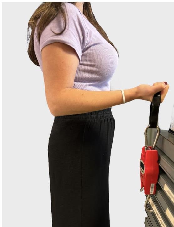
**Figure 8.1:** Estimation of Maximal Voluntary Contraction (MVC) of *biceps brachii* performing the *elbow flexion*: this is the experimental set-up followed during the measure of the MVC of each subject.
