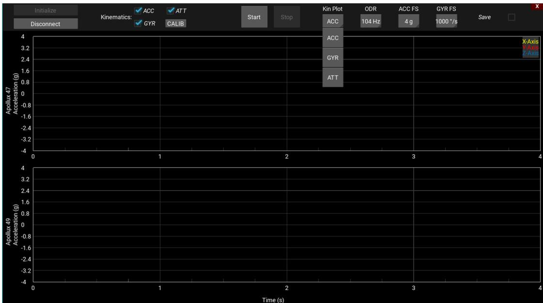
**Figure 5.3:** Previous GUI IMU: the top layer contains the widgets that allow the user to interact with the Apollux devices. The bottom contains the graphic elements that will plot the acquired data.
