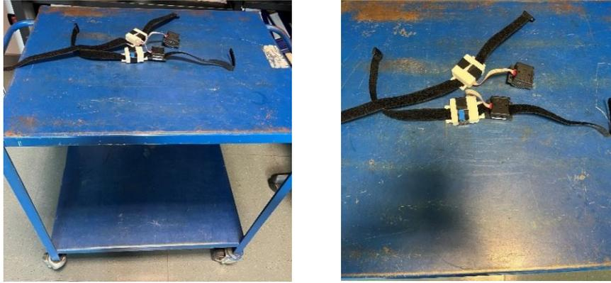
Fig.28: Set up used for Test 3. The sensors were placed at a constant height on a cart, subjected to temperature variations.
