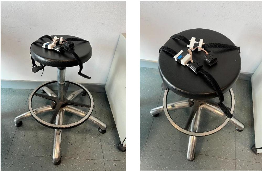
Fig. 219: Set up for *Test 1* and *Test 2*. The sensors are positioned at constant height, in static condition.
