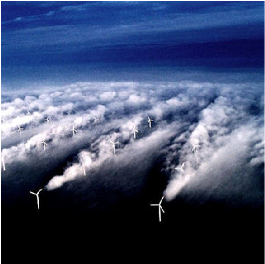
Figure 4.4: Wake interactions in Horns Rev Offshore Wind Farm, Denmark. Photo by Christian Steiness / Vattenfall
