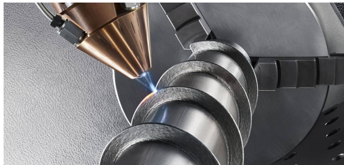
Figure 2.5. Directed Energy Deposition(source: D.E Deposition )
