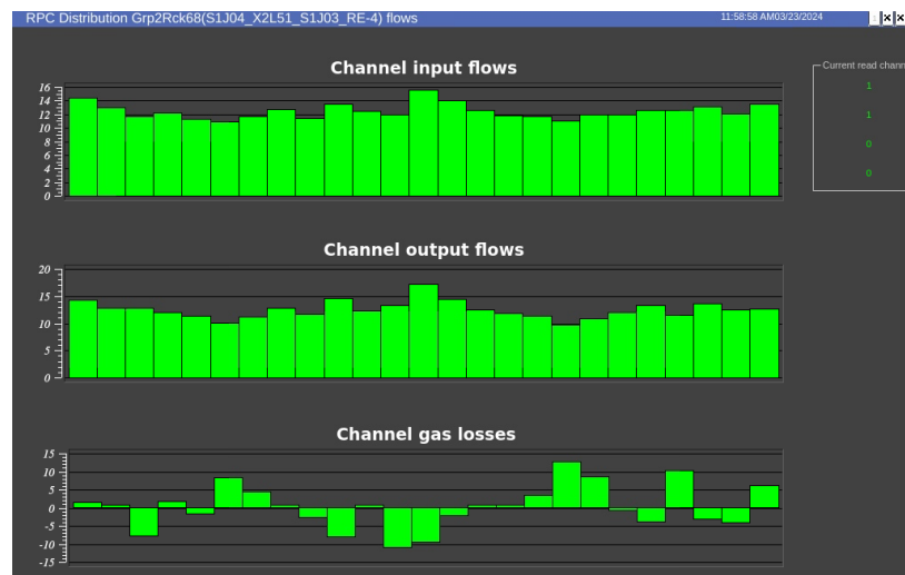
Figure 2.20: CMS RPC gas system distribution rack 68 flowcells measurements
