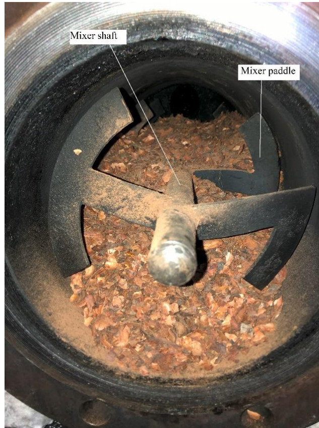
Figure 13 Internal chamber of Horizontal Unit batch reactor
