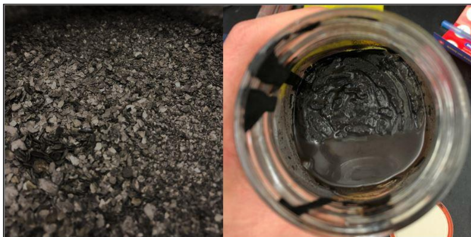
Figure 14 Solid and liquid products from slow pyrolysis of cocoa shells
