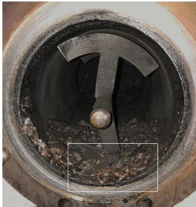
Figure 16: Detail of solid unreacted material obtained at 350°C for 1 hour
