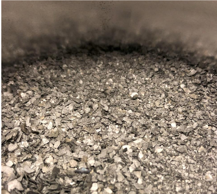
Figure 22: Biochar obtained in continuous mode at 500°C.
