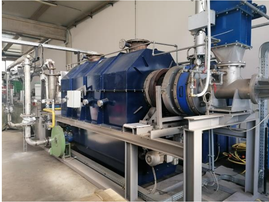
Figure 7: Rotating kiln carbonization pilot plant, capacity 100 kg/h of biomass (ReCord, n.d.).
