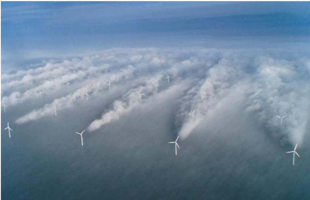
Figure 10 Wake effects visualization
