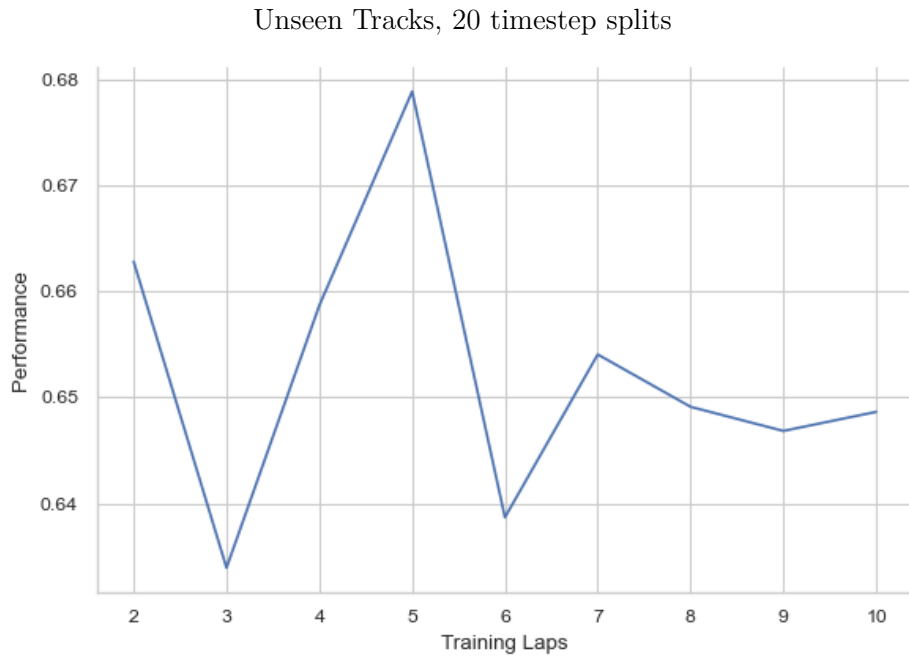
(b) Performance of the model resulting from training on Tracks 0, 1, 2 and 4 as the number of training laps increases. Evaluations performed on Track 3.
