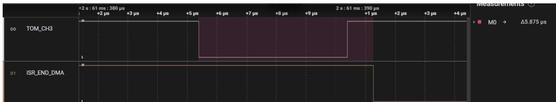
**Figure 6.22:** The time interval between the initial trigger and the conclusion of the DMA transaction is to be quantified utilising the methodology delineated in Method 2.
