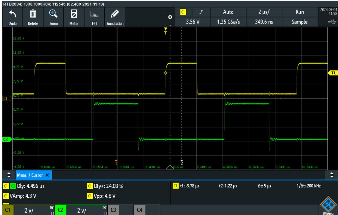
**Figure 6.15:** phase shift between **ntr1** and **ntr3** acquired by oscilloscope. From the measurements,  $\Delta t = 5 \mu\text{s}$
