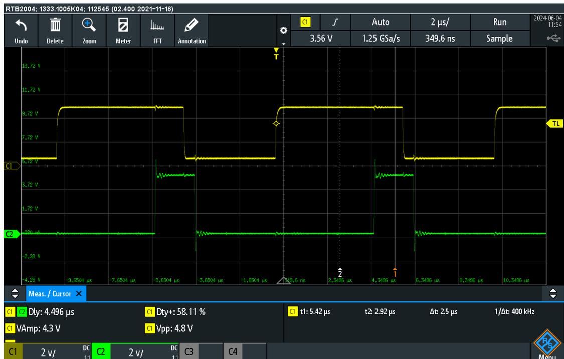
**Figure 6.14:** phase shift between **ntr1** and **ntr2** acquired by oscilloscope. From the measurements,  $\Delta t = 2.5 \mu\text{s}$
