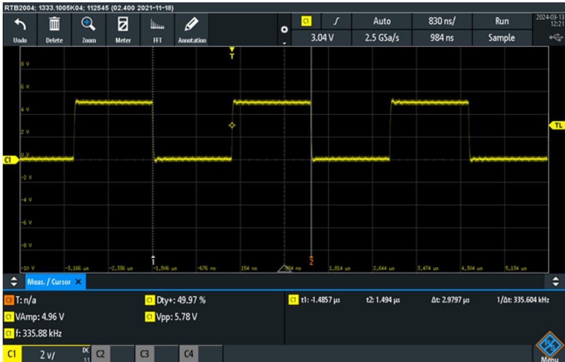
**Figure 6.11:** Output signal Produced in External Clock Output Mode when Backup Clock is active
