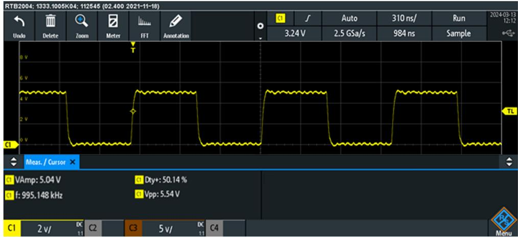
Figure 6.9: Output signal produced in External Clock Output Mode
