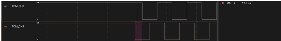
**Figure 6.20:** Representation of the trigger sequence for EVADCs from channels TOM\_CH3 and TOM\_CH4 following the first arrival of the external reset signal.
