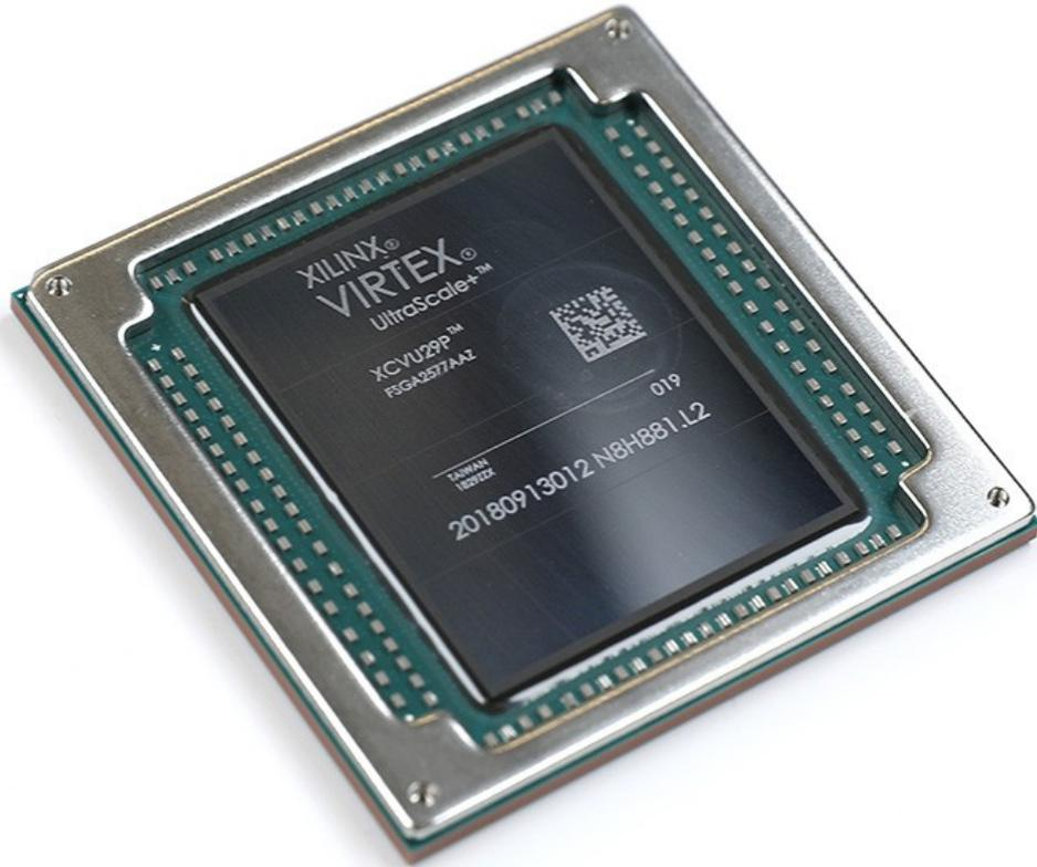
**Figura 2.1:** FPGA Virtex™ UltraScale+™
