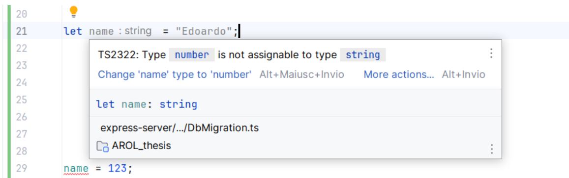
Figure 3.2: Typescript infers the 'string' type even if it's not declared and the IDE throws an error
