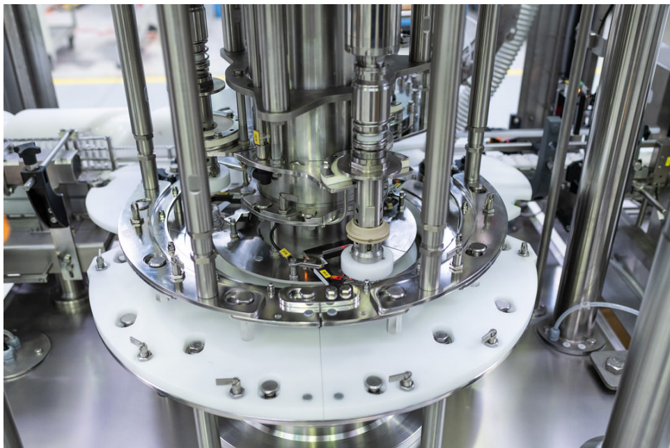
Figure 2.2: Images of AROL Equatorque capping machine [3]
