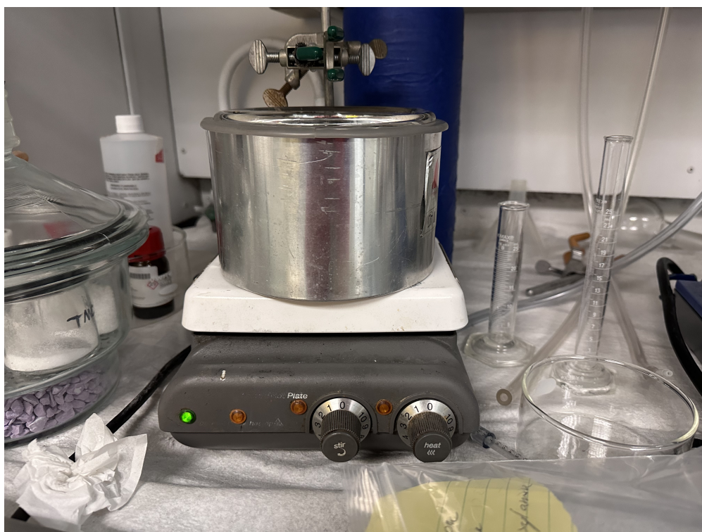
Figure 3.6: Dewar flask on magnetic plate, with clamps to hold the low temperature vial.
