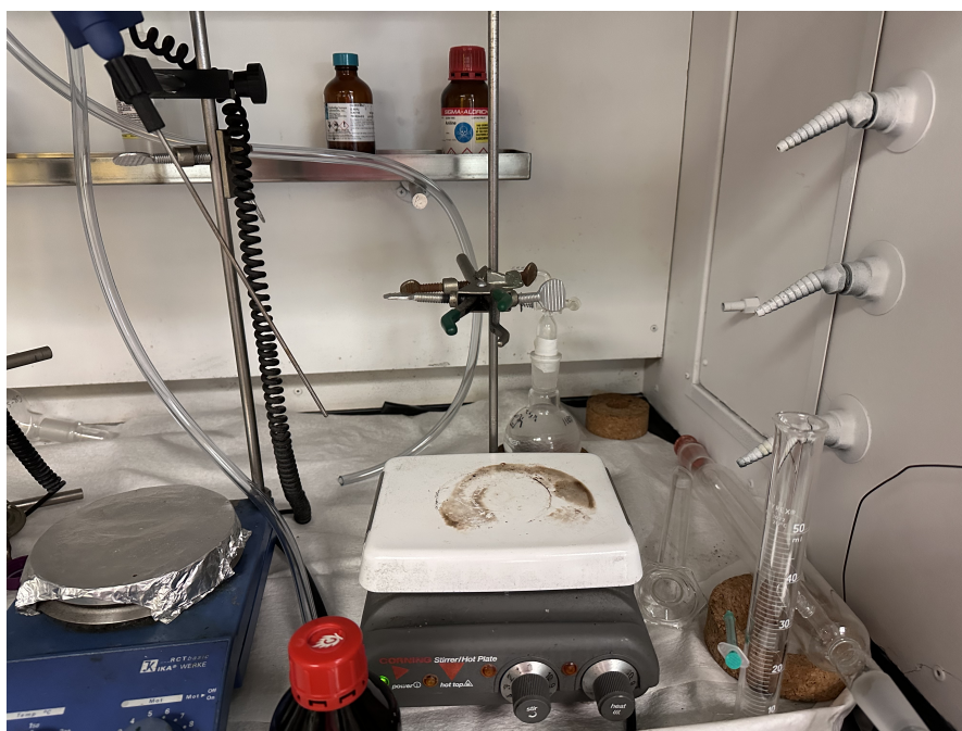
Figure 3.15: Corning™ PC-220 Pyroceram™ Hot Plate Stirrer.
