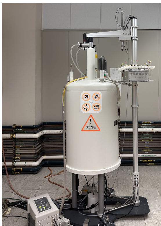
Figure 3.17: 400 MHz Bruker Avance NMR instrument.
