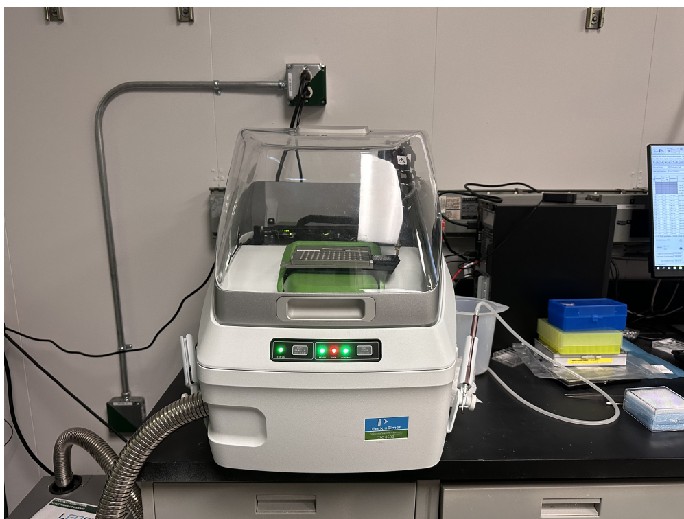
Figure 3.14: DSC 8500 Perkin Elmer machine.
