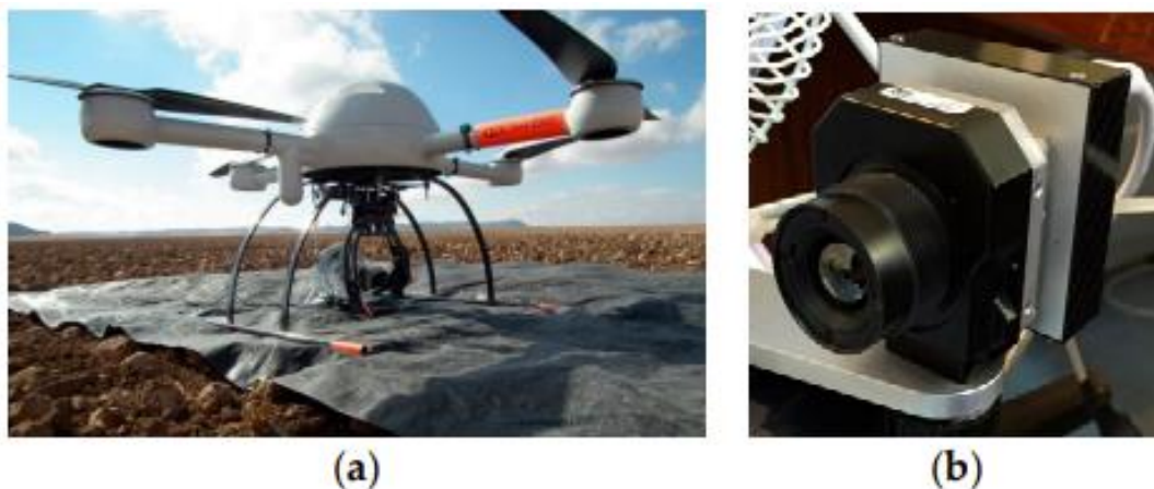
Figure 19 – (a) Unmanned aerial vehicle; (b) uncooled thermal camera [43]
