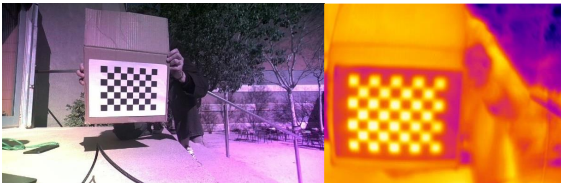
Figure 38 - Calibration process: images acquisition in the sun
