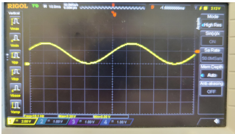
FIGURE 4.2: ESP32 16Hz Sine wave generated by the ESP32 Signal Generator software.
