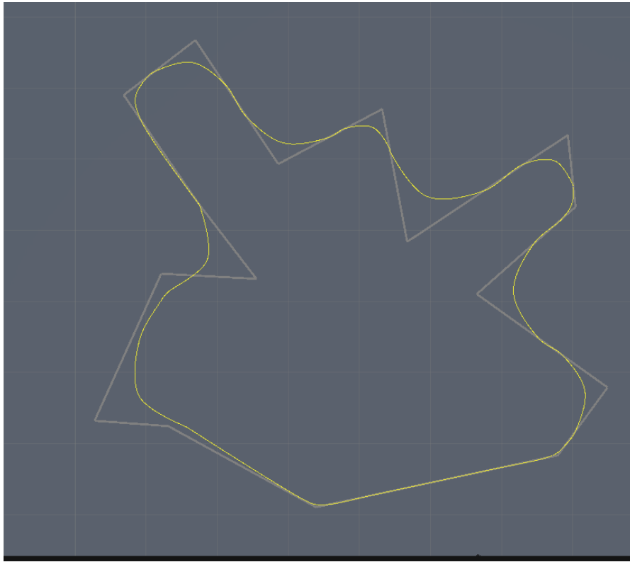
Figure 3.6: Random race track generation. White: original random polygon, Yellow: final center-line of the race track
