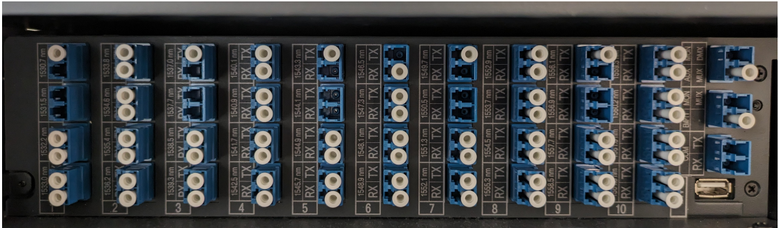
Figure 3.3: This figure represents a non-reconfigurable multiplexer provided by CISCO.
