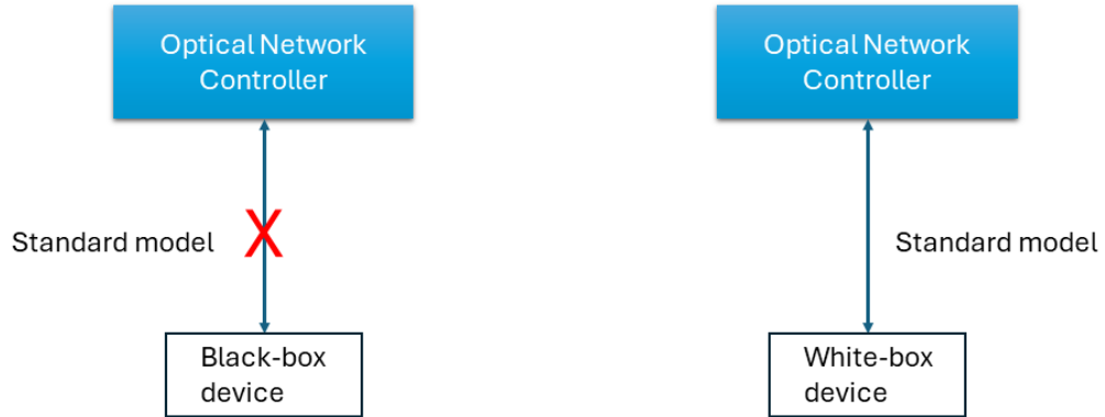
Figure 2.23: With the introduction of an open interface, a black-box device becomes accessible by the ONC, now able to use a standard model.
