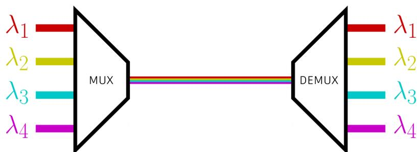
Figure 1.7: Representation of a WDM setup.
