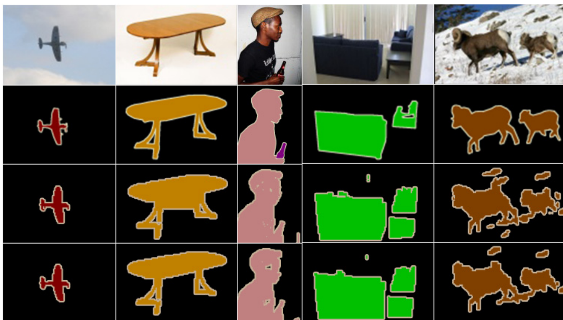
Figure 5.4: Sample segmentation results from the VOC 2007 segmentation dataset. The first two lines are the original images and ground truth. The third and fourth models use RGB color distance and LAB color distance as edge weight, respectively.
