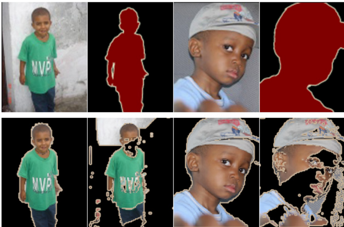
Figure 5.8: Sample segmentation results from the VOC 2007 dataset. The first row shows the original images and ground truth. The second row displays the model's segmentation results using bidirectional n-link and unidirectional n-link, respectively.
