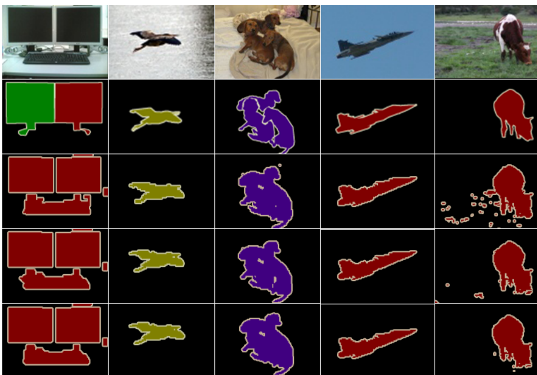
Figure 5.6: The figure illustrates segmentation outcomes from the VOC 2007 dataset. The top two rows contain the original images and the corresponding ground truth. The third, fourth, and fifth rows respectively demonstrate the model’s application of lattice, triangular, and quadrilateral configurations for edge connections.
