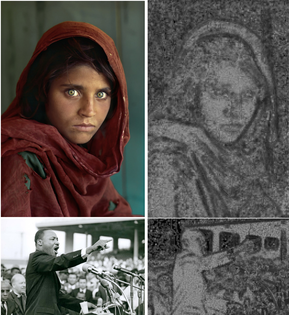
Figure 1.3: Examples of application of the FHOG algorithm. In practice, the FHOG is never used for such large images, but it is applied to a window of fixed size.
