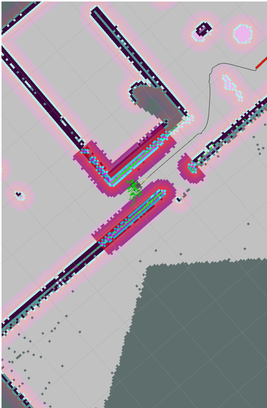
Figure 9.15: The Turtlebot creates the free-collision path, including the information sent by the Locobot
