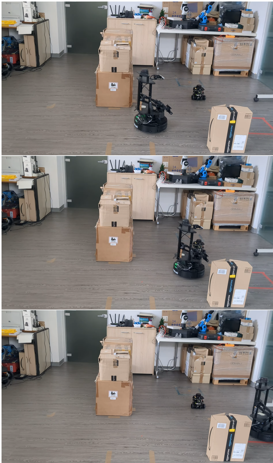
Figure 9.26: The execution of the Locobot's path, which correctly avoids the object.
