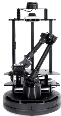
Figure 4.1: Locobot WidowX-250 6 DOF (Kobuki) [43]
