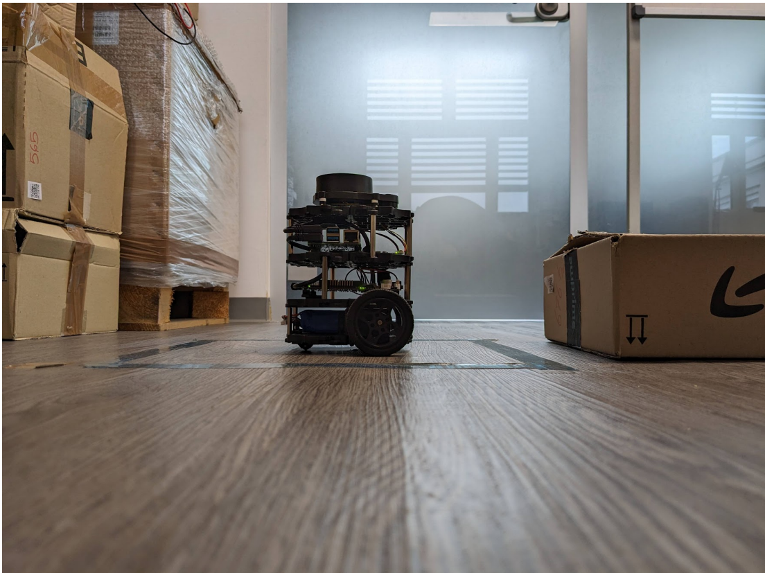
Figure 9.27: The Turtlebot LiDAR is positioned higher than the height of the box.
