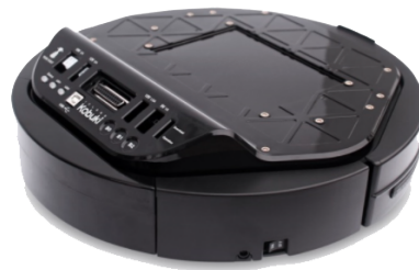
Figure 4.3: Kobuki mobile base [43]
