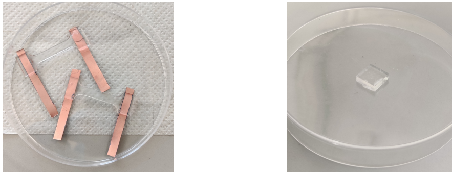
Figure 2.8: Dogbone (left) and square (right) sample of the ionic-liquid based polymer
