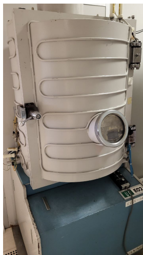
Figure 3.11: Evaporator ULVAC EBX-14D
