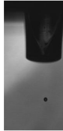
Figure 3.22: Ejection of a well-defined droplet
