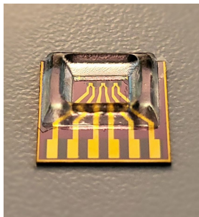
Figure 3.34: Chip with bonded PDMS chamber
