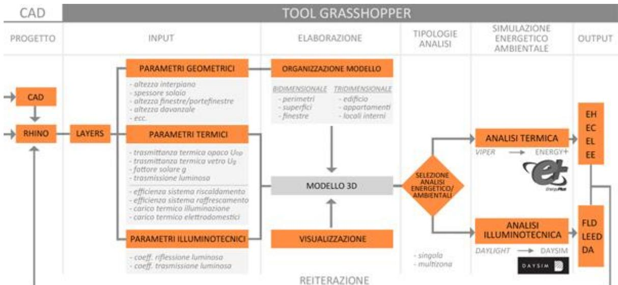
Flowchart visualizing the use of the Tool and its connection with Rhinoceros and with the energy simulation process (Energy Plus and Daysim)
