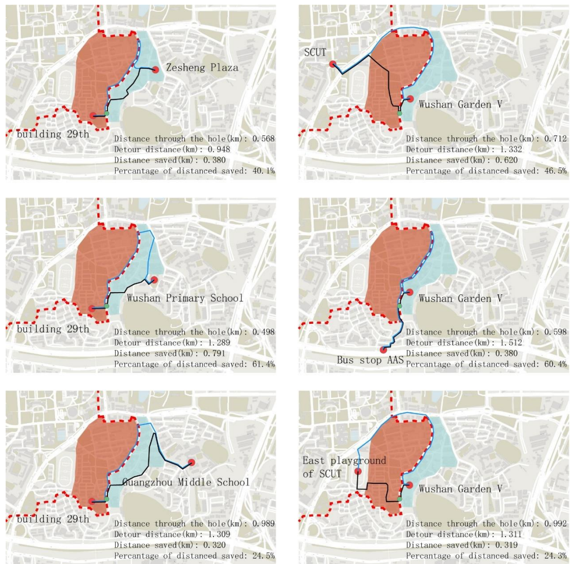
Figure 4-32 Comparison of distances between residential detours and through-hole access on both sides of the road
