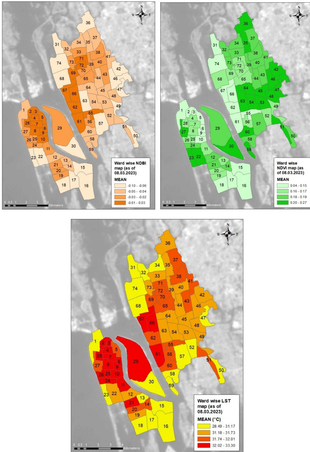
Figure 22: (On the top left) NDBI Map showing mean NDBI of each ward of KMC. (On the top right) NDVI Map showing mean NDVI of each ward of KMC. (On the bottom) LST map showing mean LST of each ward of KMC as of 08.03.2023 for comparison (Source: Author)
