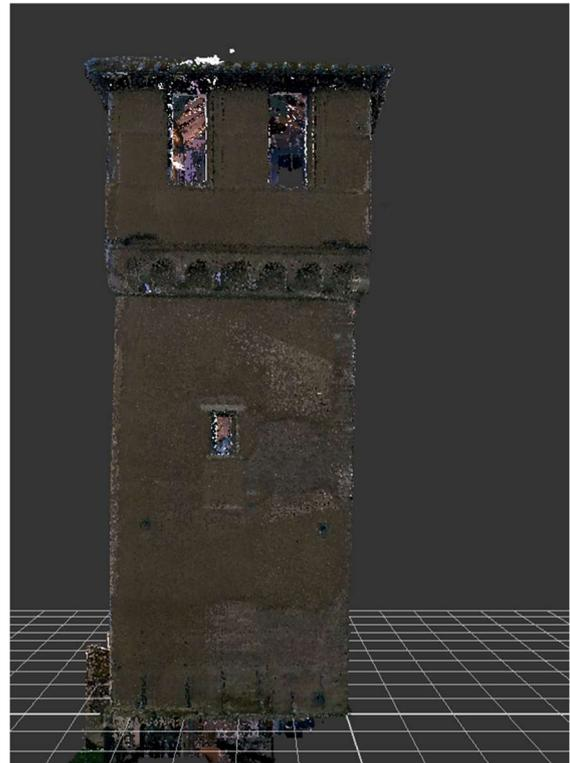
**Figure 33** Point clouds of the tower from all directions
