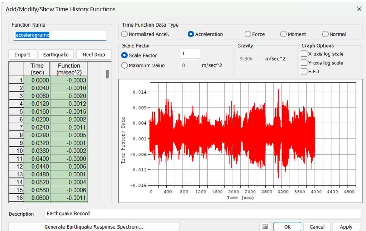
Figure 72 Accelerogram Recordings
