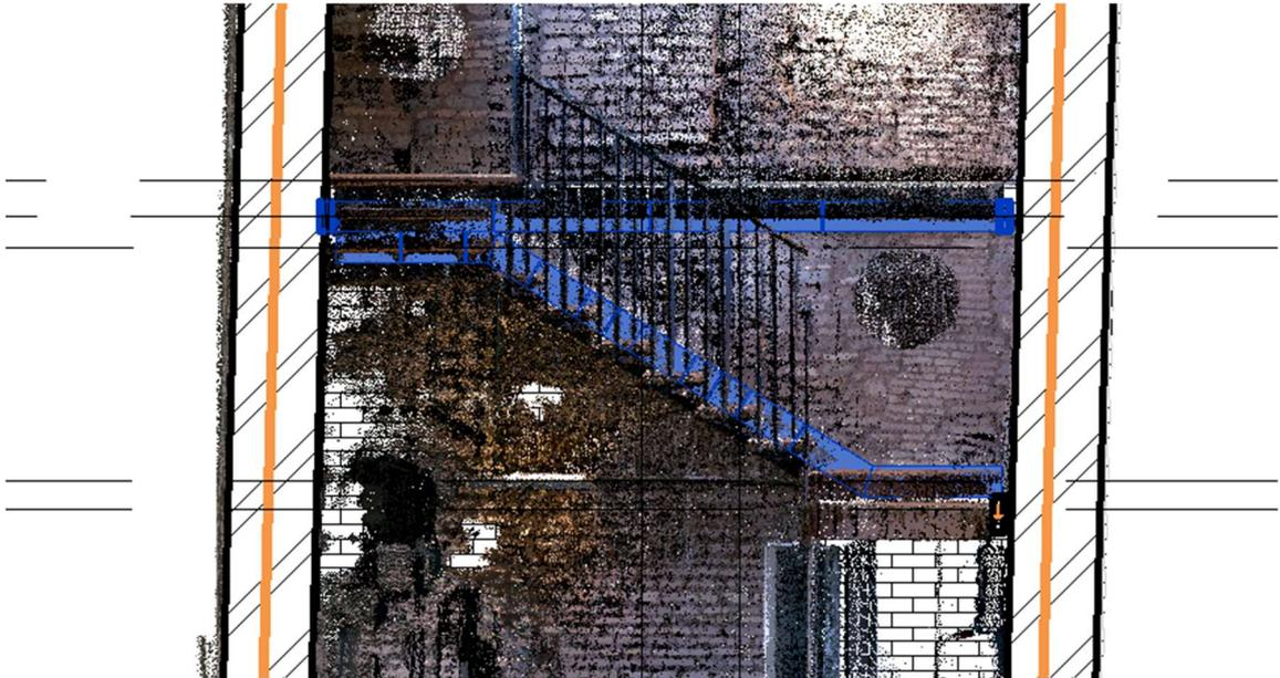
Figure 44 Beams in point cloud and aligned
