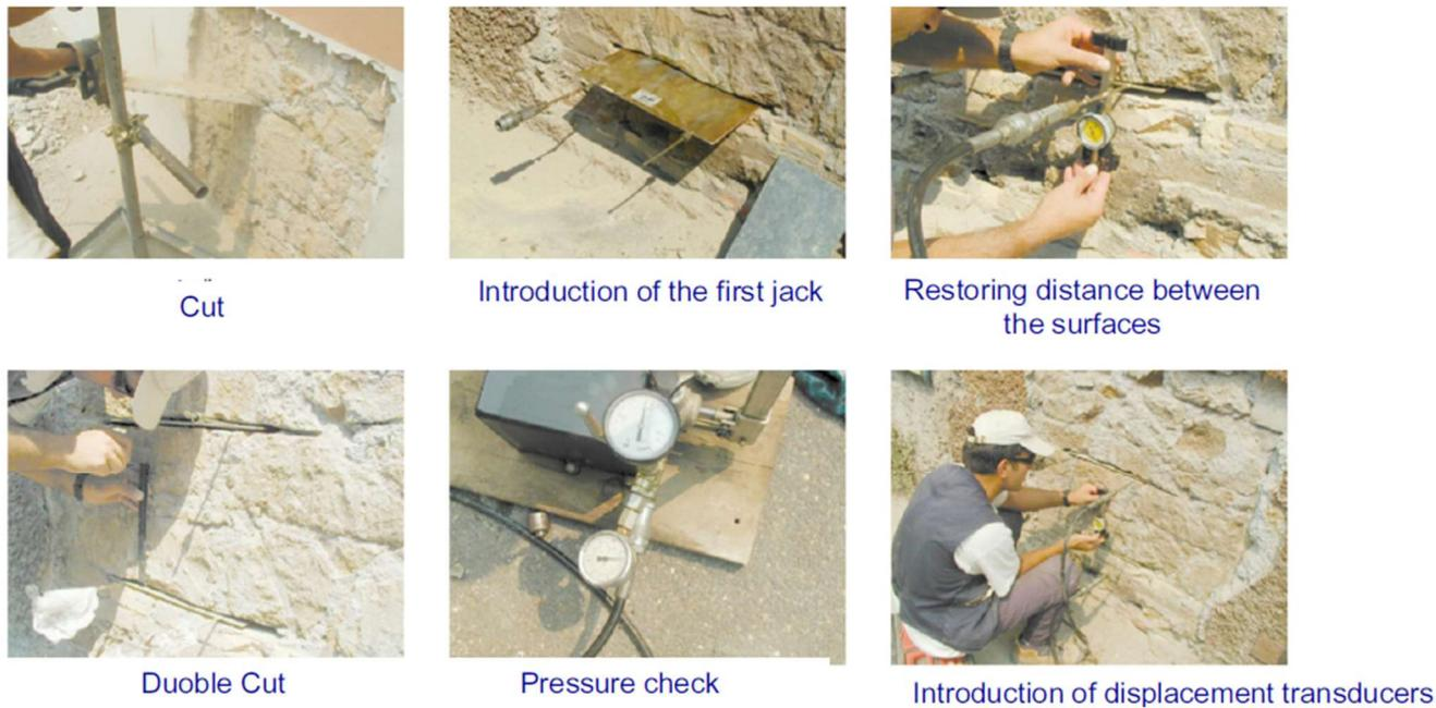
**Figure 7** Double Flat Jack test
