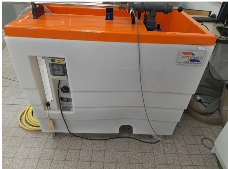
Figure 17 Water pump used to pump water in the water reservoir
