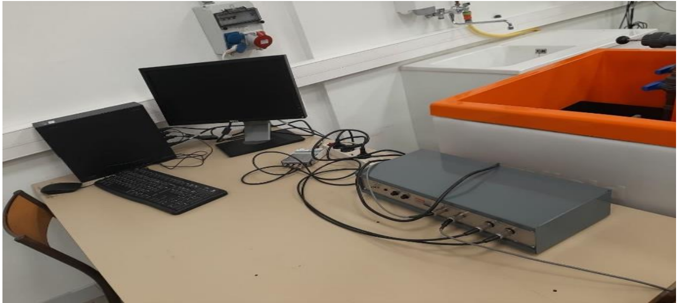
Figure 16 The computer and the receiver of the pressure sensor signals
