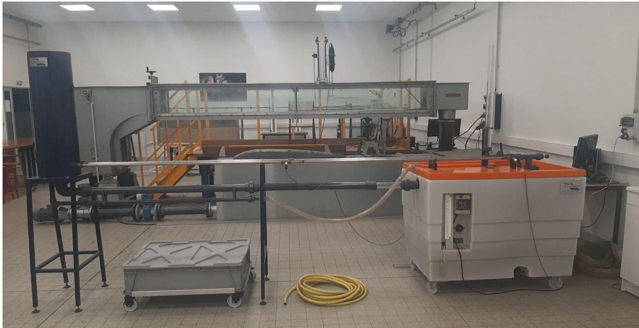
Figure 24 Water Hammer Experiment Setup in the Laboratory
