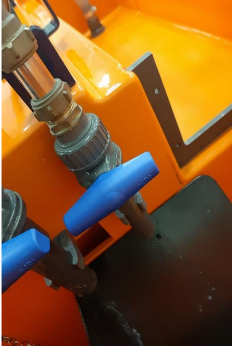
Figure 13 Keys used to control the water flow velocity
