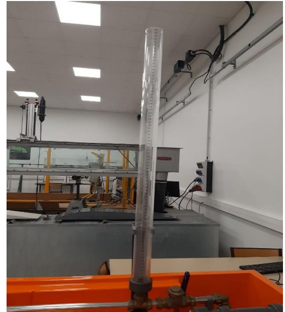
Figure 10 The Transparent Surge Shaft (equilibrium chimney)
