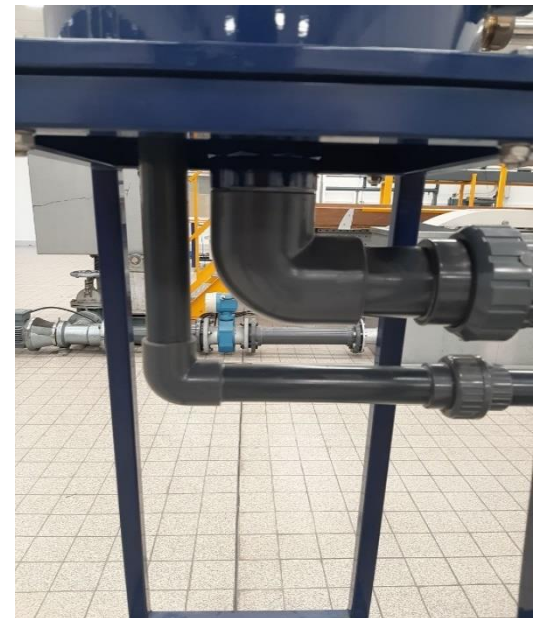
Figure 8 The inlet of the water reservoir and the outlet of the spillway
