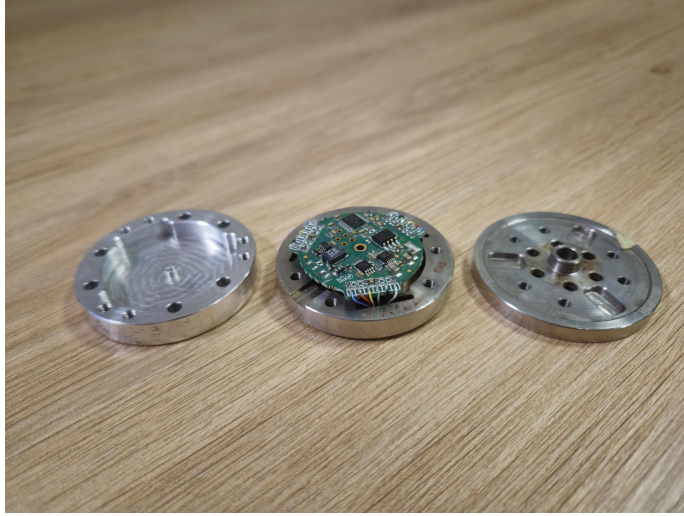
Figure 1.1: Components of 6D strain gauge force-torque sensor
