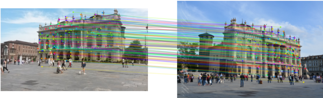
Figure 4.11: Example of keypoints extracted by SuperPoint and matched by SuperGlue. The pictures are from Turin scene train set. In the figure only 150 of the 1077 matches are shown, to have a more readable image.
