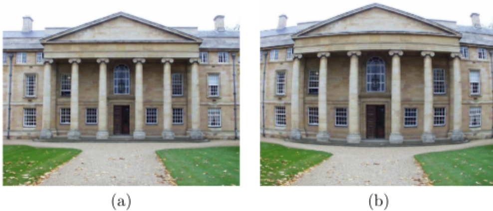
Figure 4.7: Example of radial distortion in image (b). Image (a) is the same image but undistorted.
