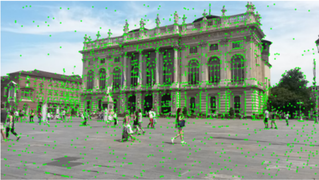
Figure 4.10: Example of keypoints extracted by SuperPoint. The picture is from Turin scene train set.
