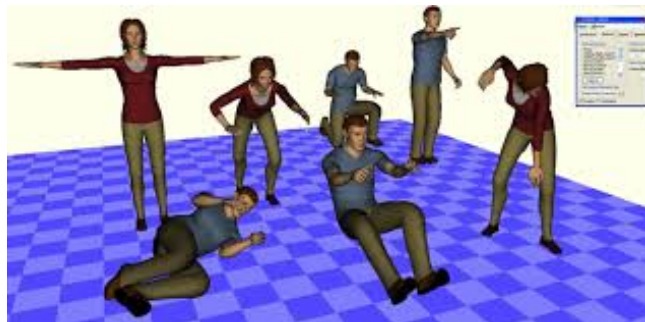
Figure 19, Jack has a library of many postures and additional postures can be easily added.
