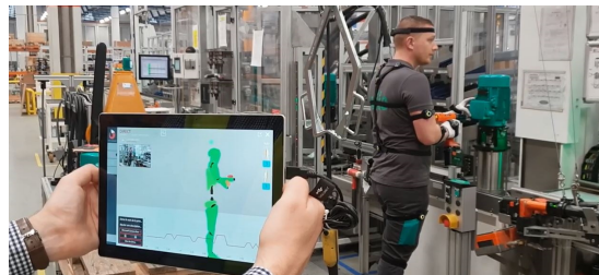
Figure 47, Mocap application in assembly line
