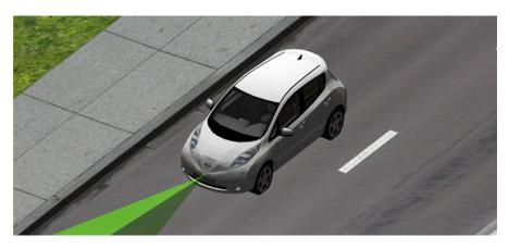
Figure 2.9: Zoomed view of radar sensor placement.
