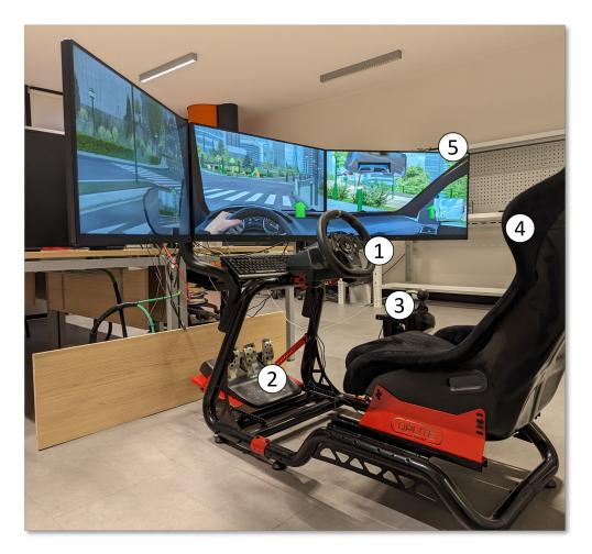
**Figure 1.1:** Driving simulator paired with SCANeR<sup>TM</sup>Studio. 1: force feedback steering wheel, 2: pedals, 3: manual gearbox, 4: bucket seat, 5: high resolution screens.
