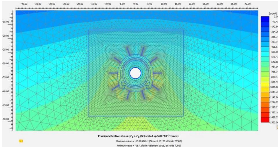
Figure 23: Isotropic Effective Stress Distribution After 5 Days of Drains Activation
