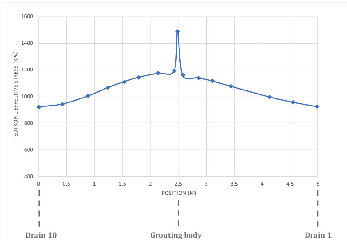
Figure 28: Isotropic Effective Stress Variation Along the Line Joining Two Drains After 5 Days ( $k = 10^{-7} \text{m/s}$ )
