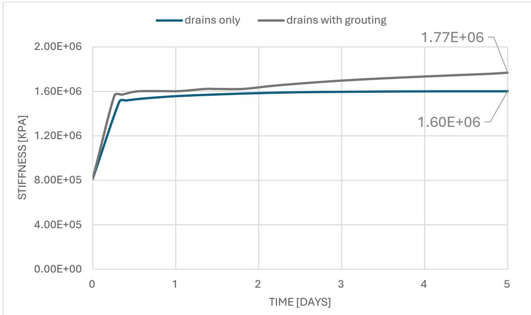
Figure 35: Stiffness Variation Over Time for The Two Case Scenarios ( $k = 10^{-7} \text{ m/s}$ )
