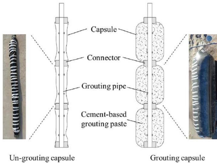
Figure 7: Schematic Diagram of Capsule Grouting Technology (CGT) (Zheng et al., 2021)
