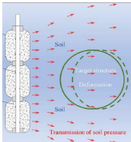
Figure 8: Mechanism of Soil Pressure Transmission and Deformation Control using CGT (Zheng et al., 2022)
