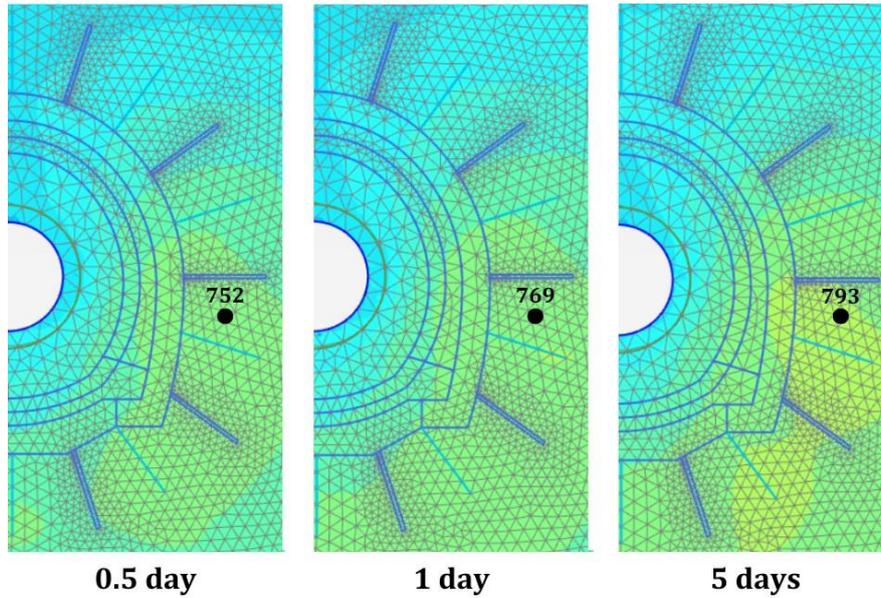
Figure 26: Isotropic Effective Stress Distribution for The Drains Only Case at 0.5 Day, 1 Day, and 5 Days
