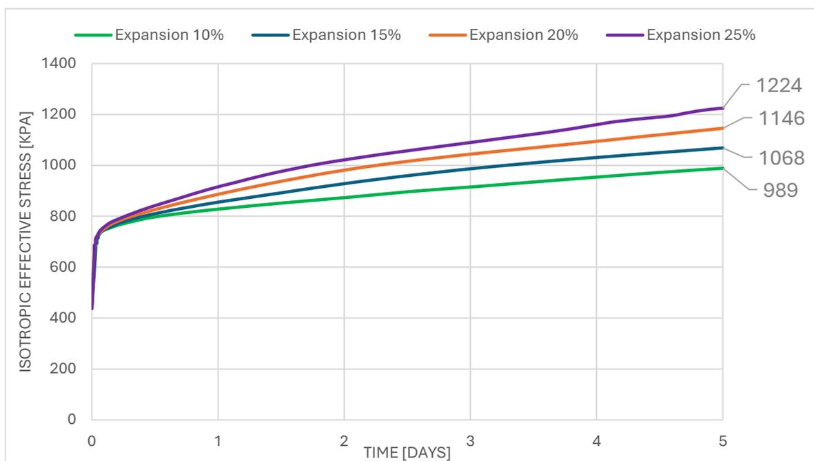
**Figure 40: Isotropic Effective Stress Variation Over Time for Different Volumetric Expansions in Grouting ( $k = 10^{-7} \text{m/s}$ )**
