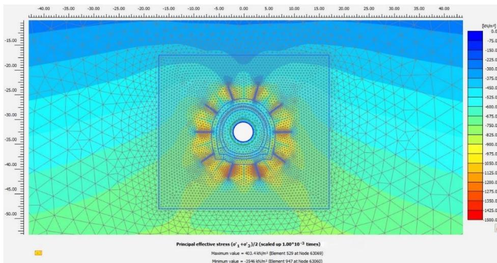
Figure 24: Isotropic Effective Stress Distribution After 5 Days of Drains and Grouting Activation
