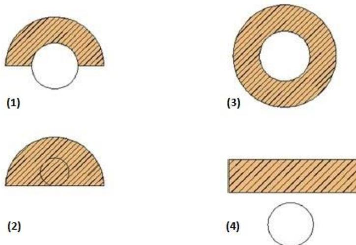
Figure 5: Example of Grouting Profiles (Kogler, 2013)
