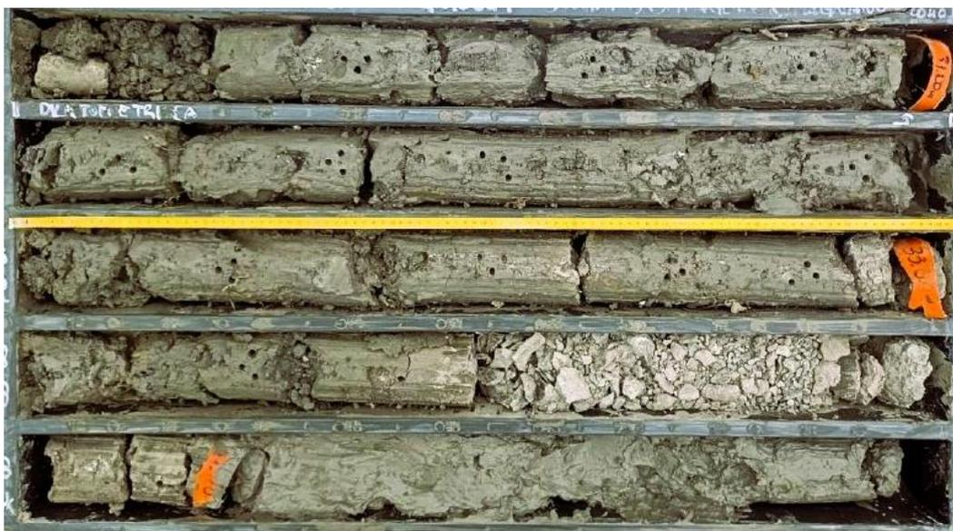
**Figure 15: Cores From 30 to 35 meters in the Borehole Showing the Mixed Formation in its Fine-Grained Component**
