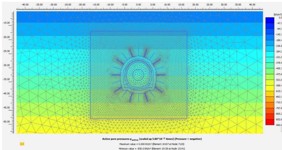
Figure 29: Active Pore Water Pressure Distribution in the Initial State
