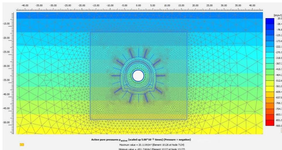
Figure 30: Active Pore Water Pressure Distribution after TBM Section Construction
