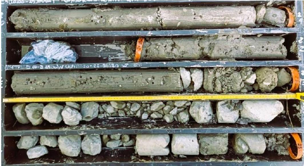
Figure 16: Cores From 20 to 25 meters in the Borehole Showing the Mixed Formation in its Coarse Component
