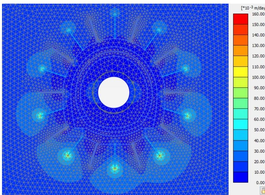
Figure 34: Groundwater flow  $|q|$  Distribution after Drains and Grouting Activation
