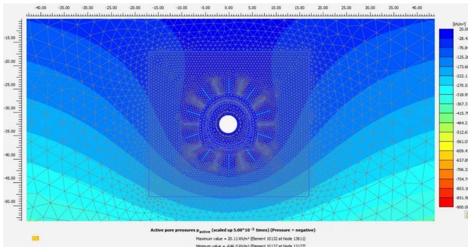
Figure 32: Active Pore Water Pressure Distribution After 5 Days of Drains and Grouting Activation
