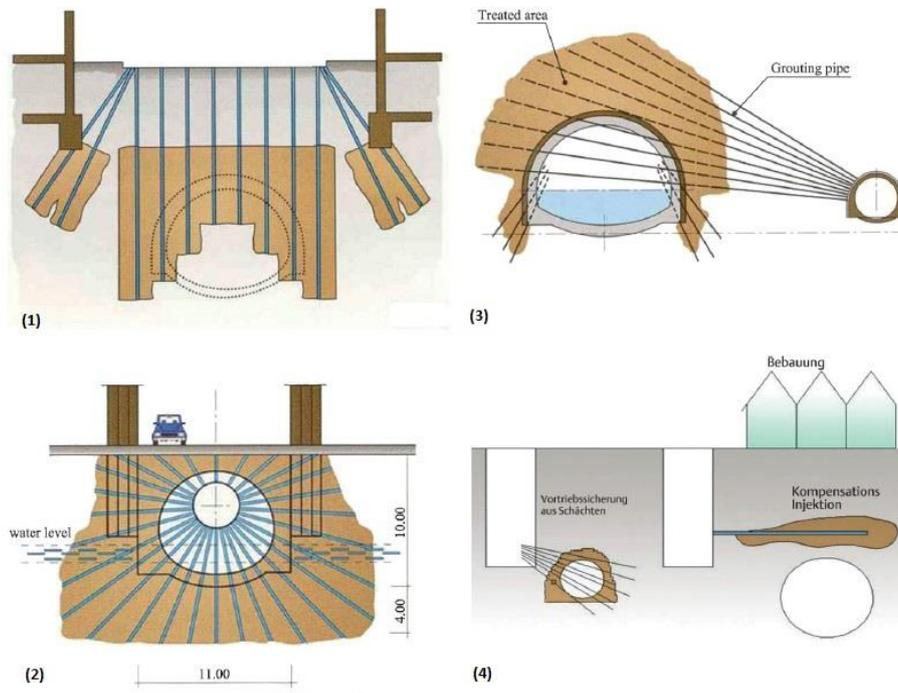
Figure 6: Drilling works: (1) from surface; (2) from adjacent gallery; (3) from pilot gallery; (4) from shafts (Kogler, 2013)
