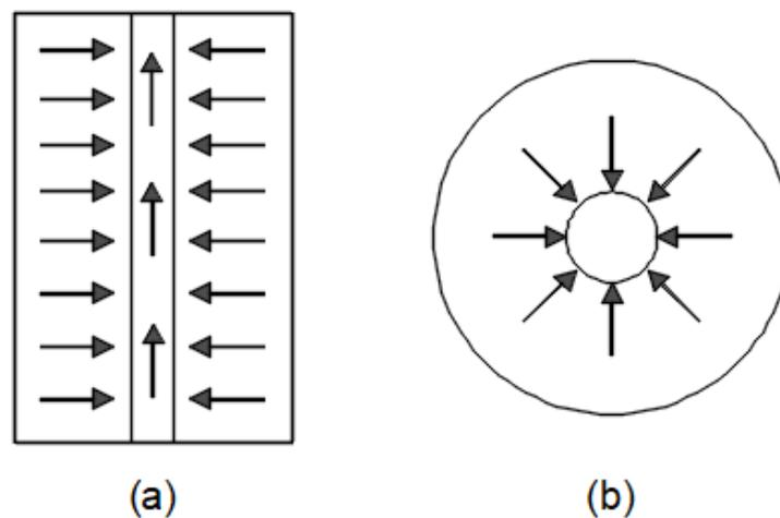
Figure 3: (a) Plane Strain (b) Axisymmetric
