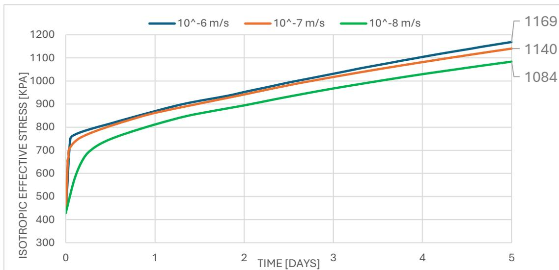
Figure 39: Isotropic Effective Stress Variation Over Time for Different Permeability values
