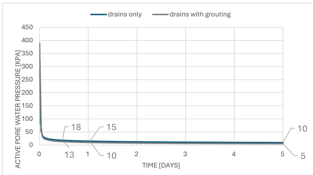
Figure 33: Active Pore Water Pressure Variation Over Time for The Two Case Scenarios ( $k = 10^{-7} \text{m/s}$ )
