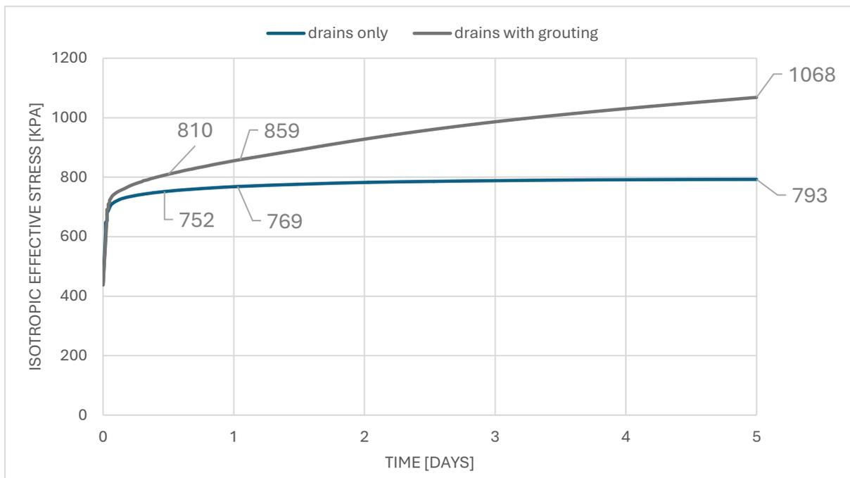
Figure 25: Isotropic Effective Stress Variation Over Time for The Two Case Scenarios ( $k = 10^{-7} \text{m/s}$ )
