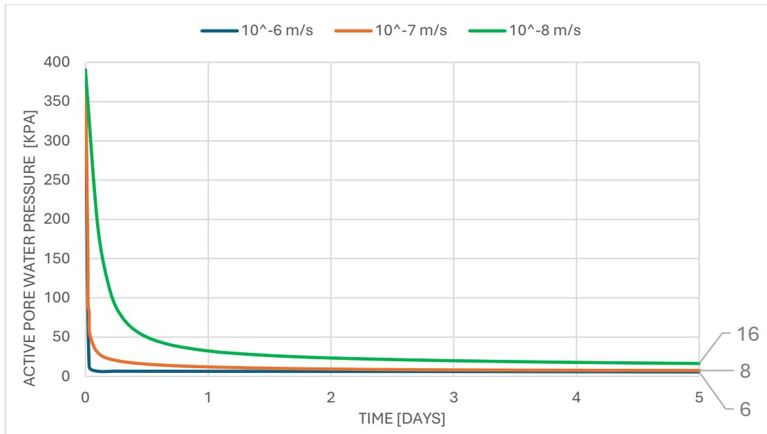
Figure 38: Active Pore Water Pressure Variation Over Time for Different Permeability values
