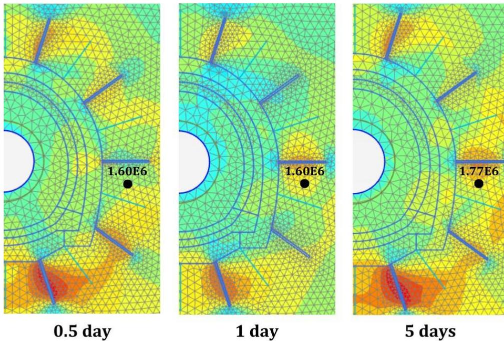
Figure 37: Stiffness Distribution for The Drains with Grouting Only Case at 0.5 Day, 1 Day, and 5 Days
