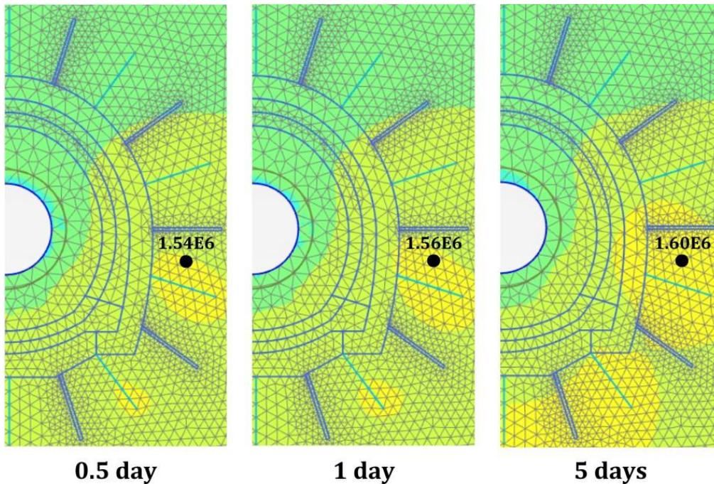
Figure 36: Stiffness Distribution for The Drains Only Case at 0.5 Day, 1 Day, and 5 Days
