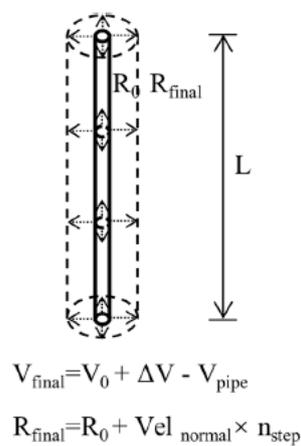
Figure 9: Principle of Capsule Grouting (Zheng et al., 2022)
