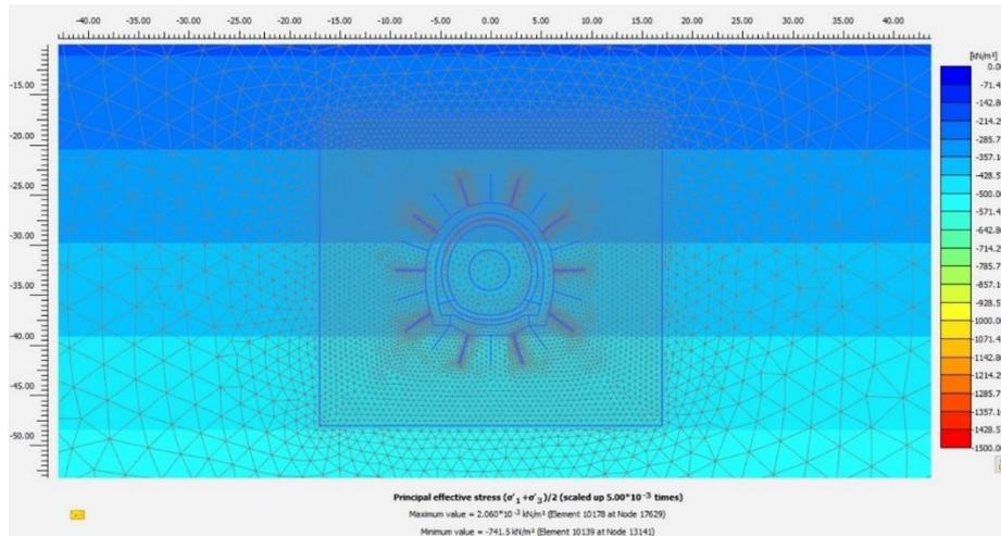
Figure 21: Isotropic Effective Stress Distribution in the Initial State
