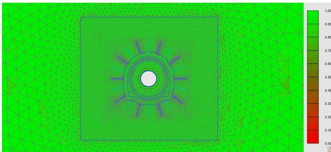
**Figure 18: Finite Element Mesh for Numerical Model**
