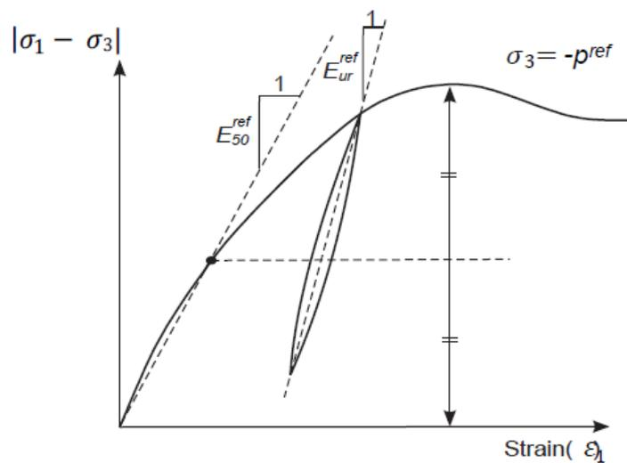
Figure 11: Definitions of  $E_{50}^{ref}$  and  $E_{ur}^{ref}$  for drained triaxial test results (Plaxis, 2023)
