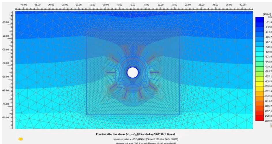
Figure 22: Isotropic Effective Stress Distribution after TBM Section Construction
