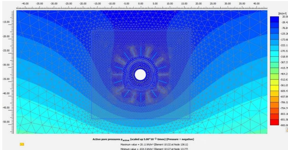
Figure 31: Active Pore Water Pressure Distribution After 5 Days of Drains Activation
