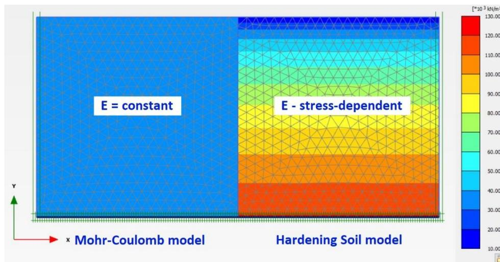
Figure 12: Comparison of Young's Modulus Variation: Mohr-Coulomb Model vs. Hardening Soil Model
