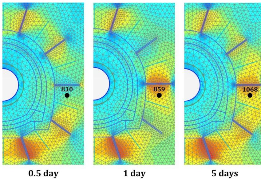
Figure 27: Isotropic Effective Stress Distribution for The Drains with Grouting Only Case at 0.5 Day, 1 Day, and 5 Days
