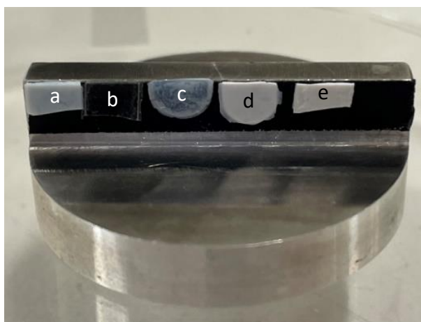
Figure 2.9. SEM stub with the cryo-fractured samples aligned, a) BMA-E45, b) BA2-E45, c) BA1-E45, d) BMA-co-BA2-E45 and e) BMA-co-BA1-E45.
