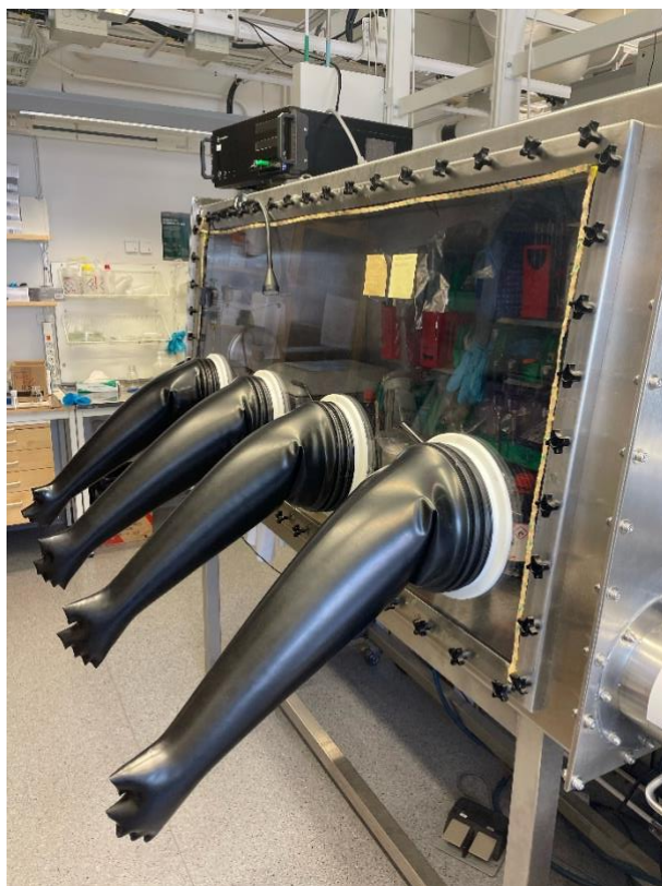
Figure 2.3. Glovebox for the synthesis in a protected atmosphere.
