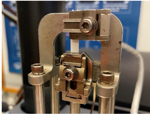
Figure 2.8. Sample installation on the DMA instrument.
