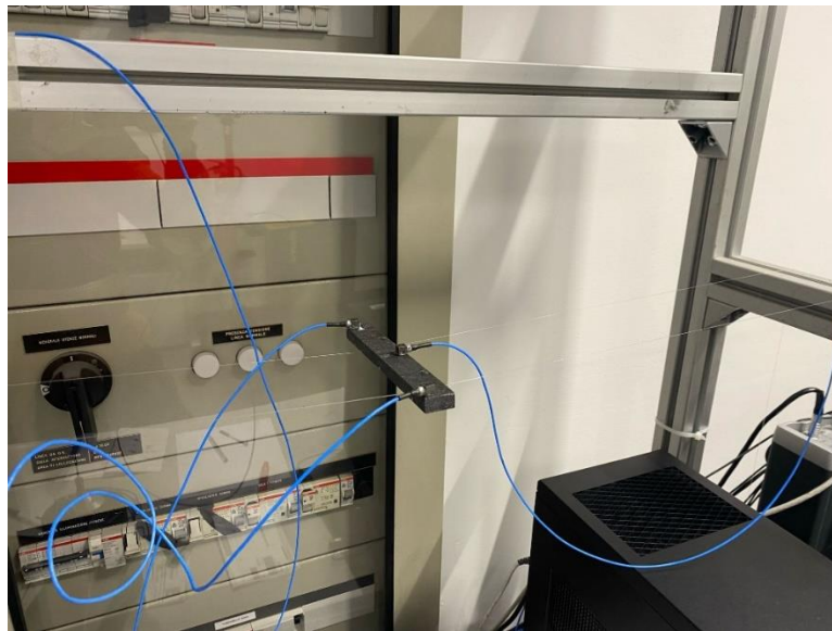
Figure 4.35. Accelerometers (blu wires) used in IET RT set up in BSCCB laboratory.
