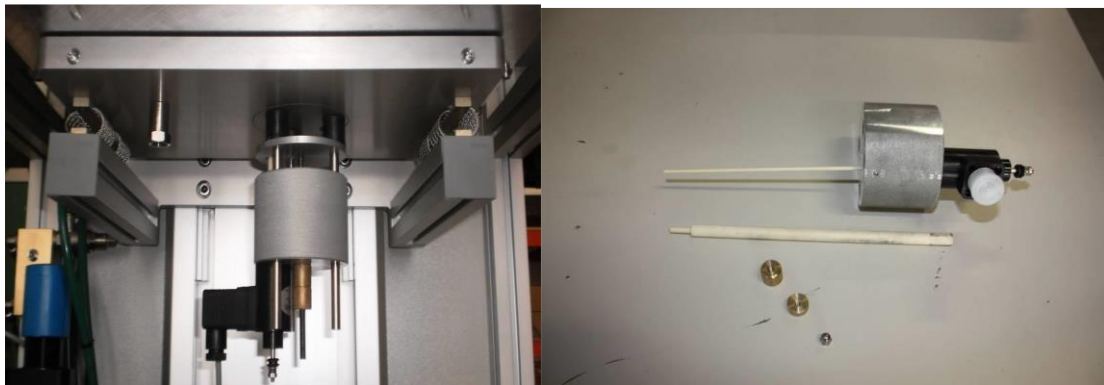
Figure 4.8. Solicitation system in situ (left) and the single components of the solicitation system: load cell, loading projectile, and alumina guide (right) [17].
