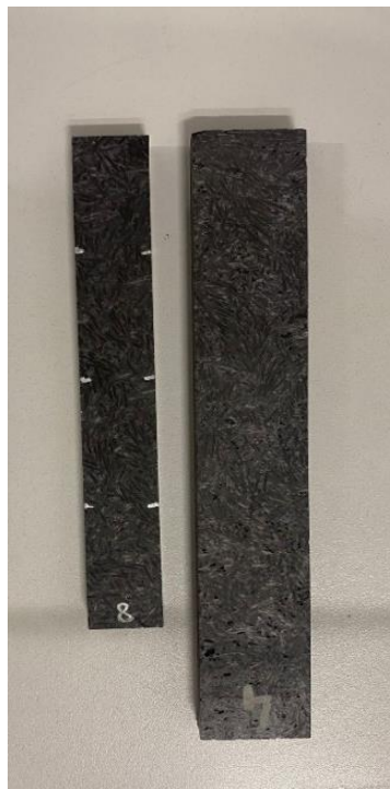
Figure 4.12. Small geometry samples (160x20x10 mm) (left); big geometry samples (200x30x12 mm) (right).
