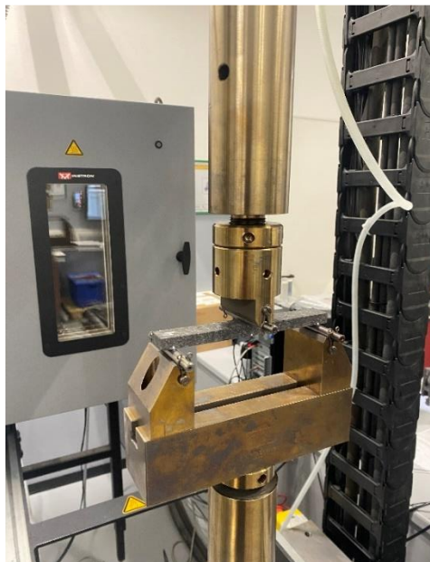
Figure 6.4. Set up of DMA 3-point bending test at room temperature with Instron 8802.
