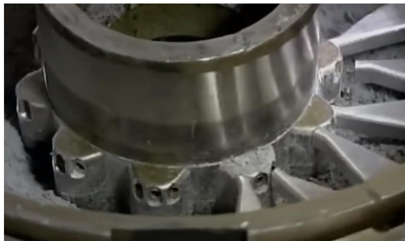
Figure 3.5. Insertion of aluminum cores to create the ventilation channels [15].
