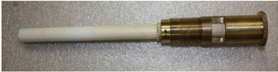
Figure 4.9. Alumina guide inside which the microphone is inserted [17].
