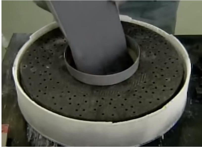
Figure 3.9. Introduction of silicon powder into the crucible [15].
