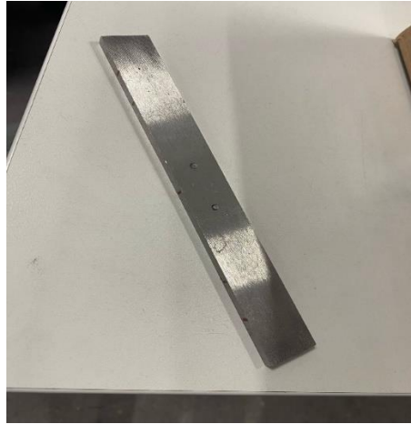
Figure 5.5. Steel bar tested with 3PB.
