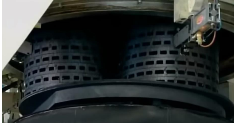
Figure 3.7. Pyrolysis treatment in the oven [15].
