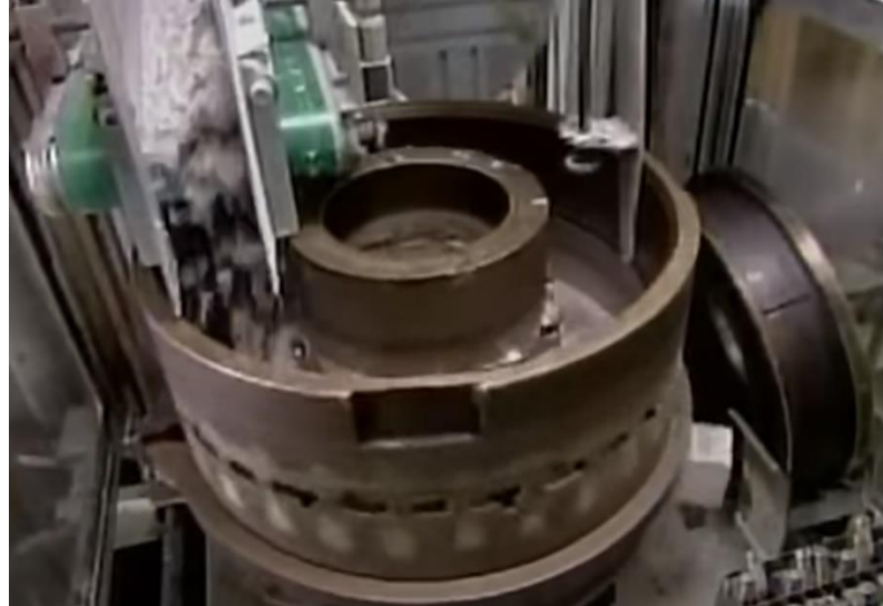
Figure 3.4. Introduction of the resin-fiber mixture into the mold [15].
