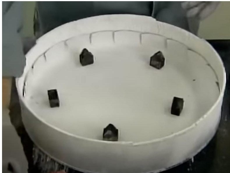
Figure 3.8. Alumina crucible used for the silicon infiltration phase [15].
