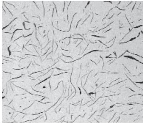
Figure 3.3. Picture of a common gray cast iron internal microstructure [10].
