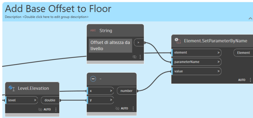
Figure 45. Add Base Offset to Floor.
