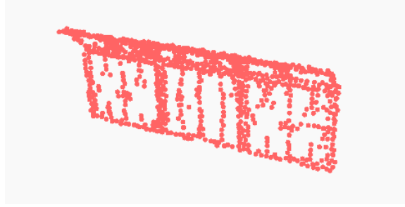
Figure 149. Window Instance Segmentation by using 3D Clustering – Chapel XXVIII.
