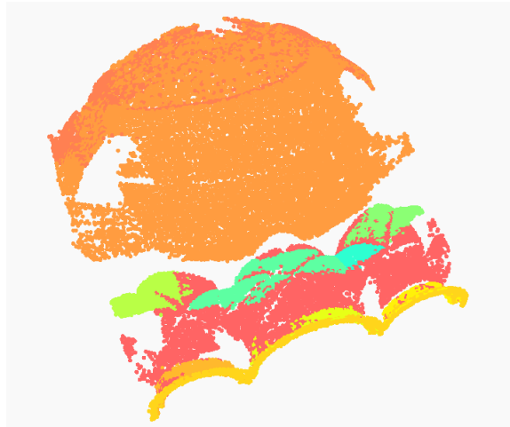
Figure 130. Vault Instance Segmentation by using 6D Clustering – Chapel XXIV.
