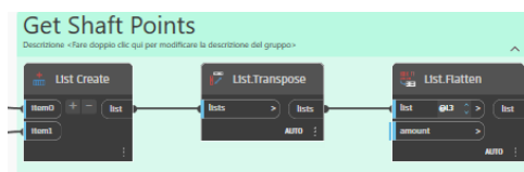
Figure 107. Selection of shaft section of column points.
