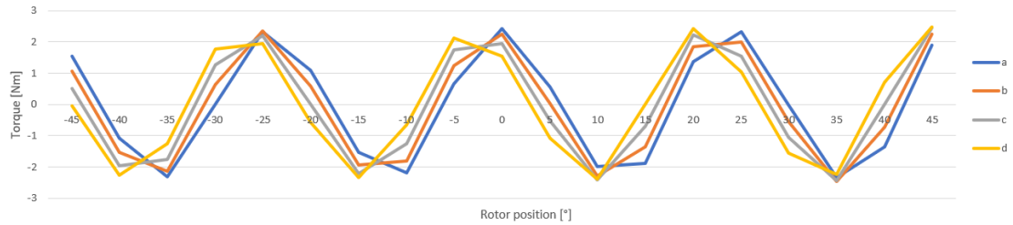
Figure 2.7: Detail of the torque generated for different moments and rotor positions
