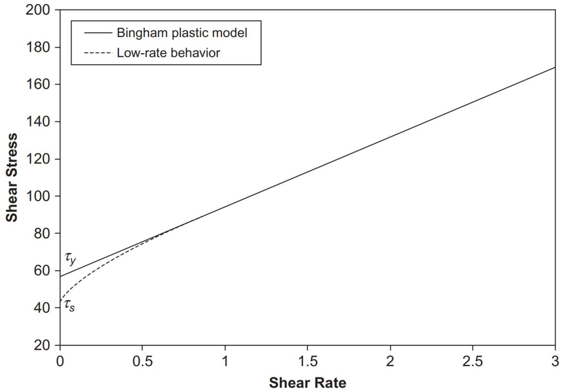
Figure 10 Bingham Model in low shear rate region (52)
