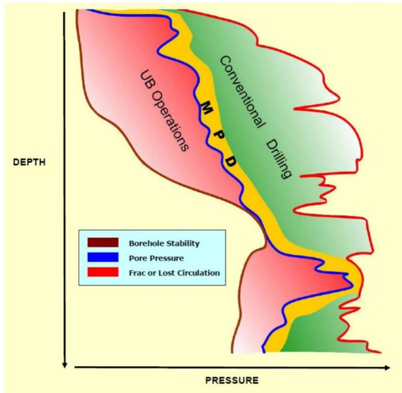
Figure 1 Mud Window for Different Drilling Methods (18)
