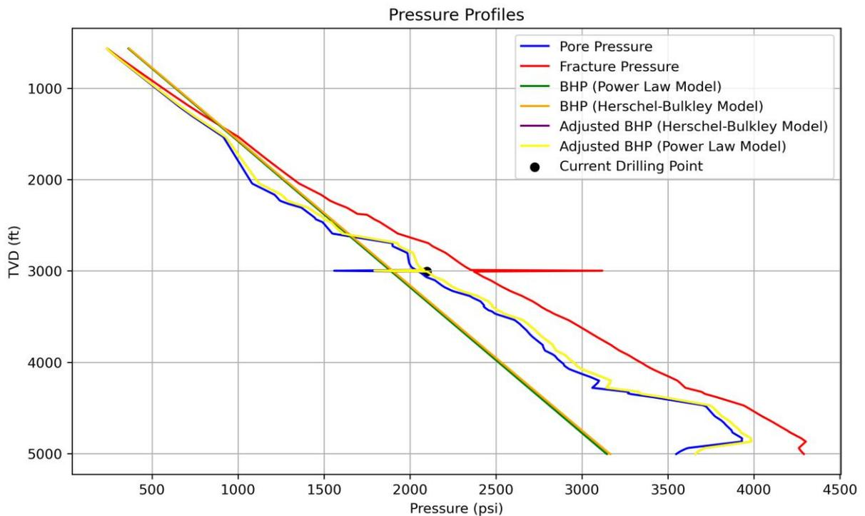
Figure 23 Real-Time Pressure Profiles
