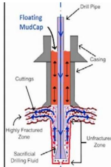
Figure 6 FMCD Schematic (37)
