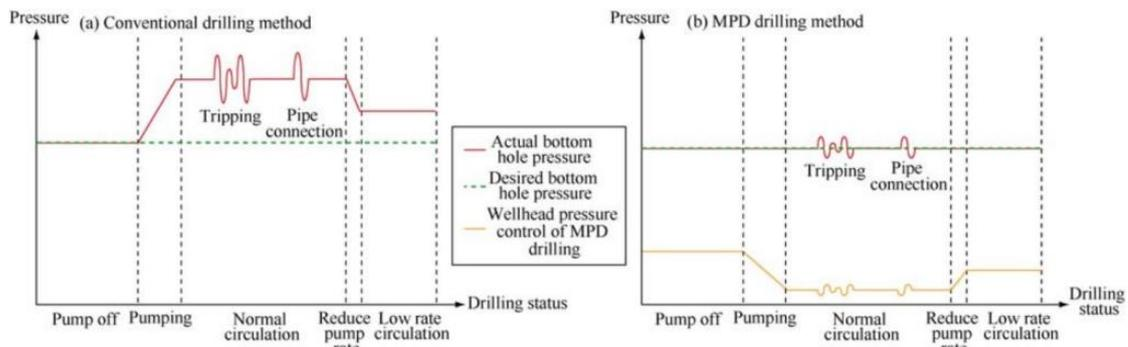
Figure 3 Conventional and MPD Drilling BHP Comparison (21)
