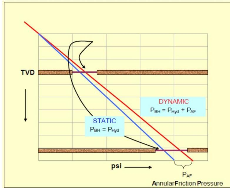
Figure 2 Dynamic and Static Pressure Profiles (18)
