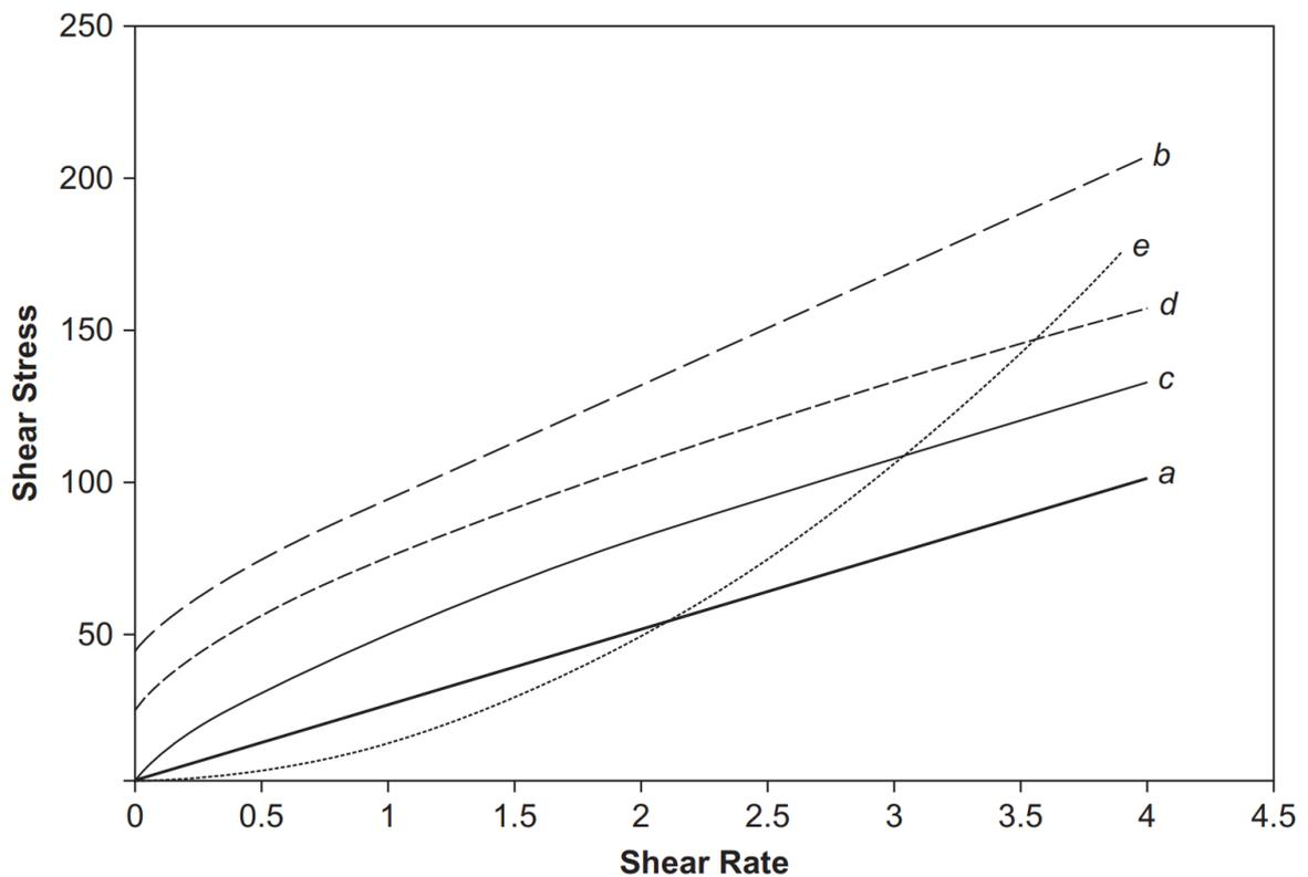
Figure 9 Fluid Types Used in Drilling (52)
