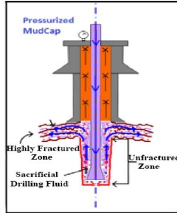
Figure 5 PMDC Schematic (37)
