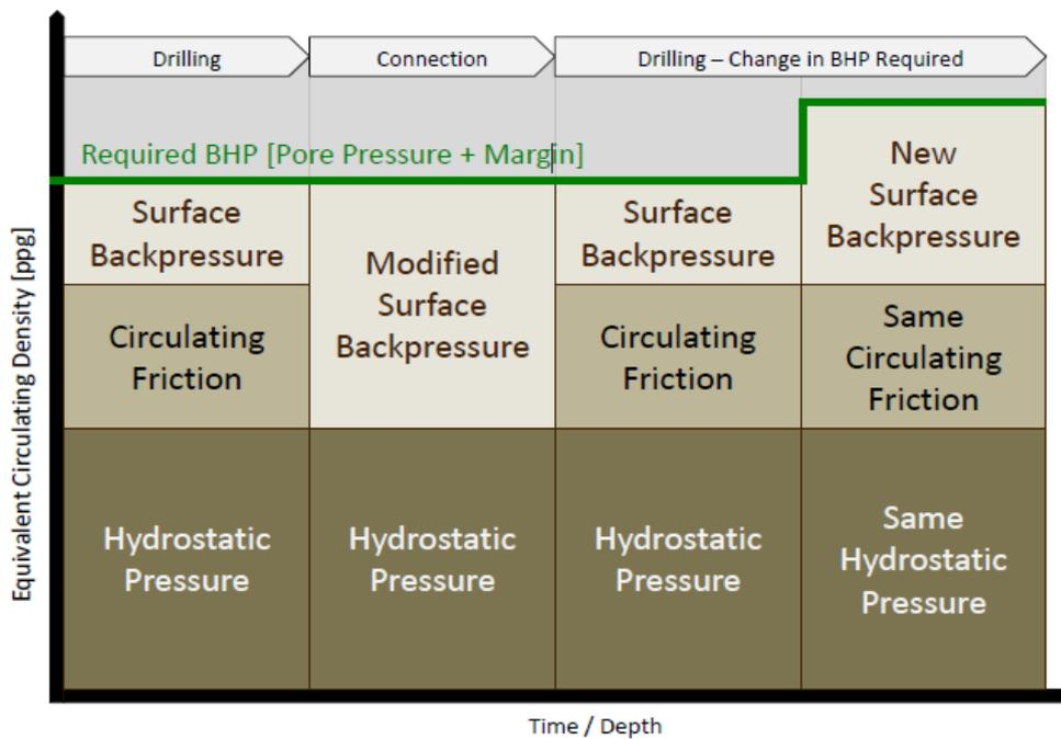
Figure 4 ECD compensation during connection with MPD (32)
