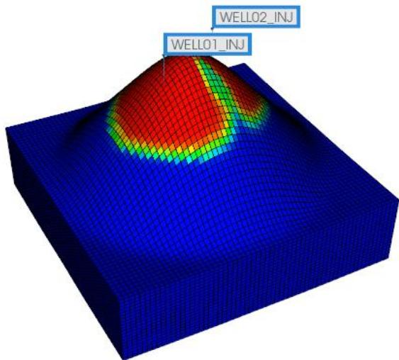
Figure 18 3D representation of model A after CO<sub>2</sub> injection
