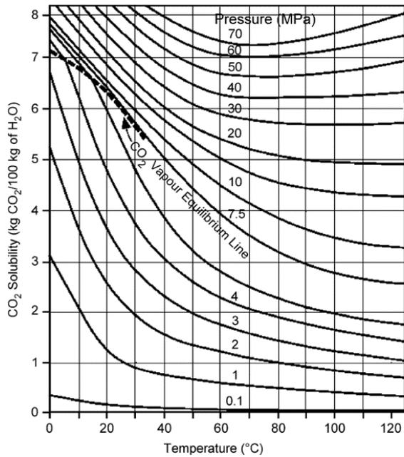
Figure 13 CO<sub>2</sub> solubility in function of pressure and temperature [22]
