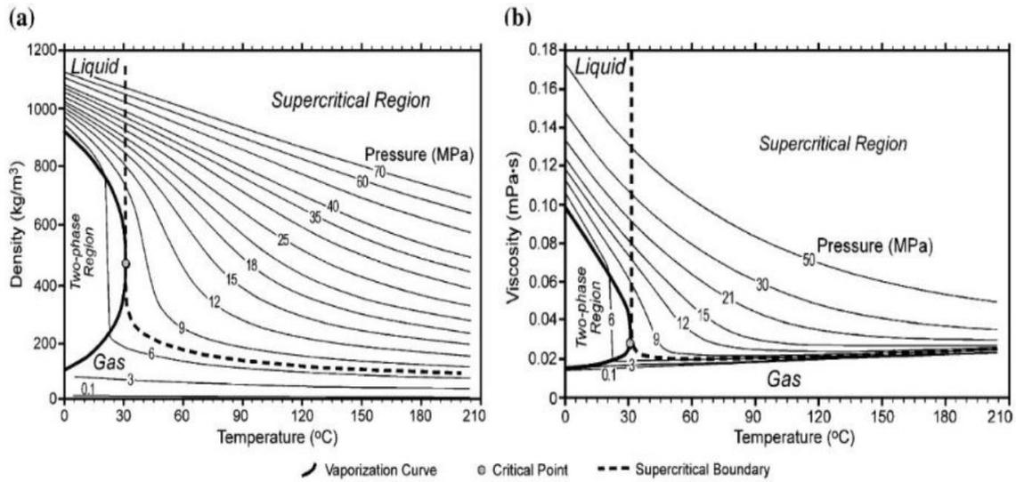
Figure 12 CO<sub>2</sub> density and viscosity in function of Pressure and Temperature [22]
