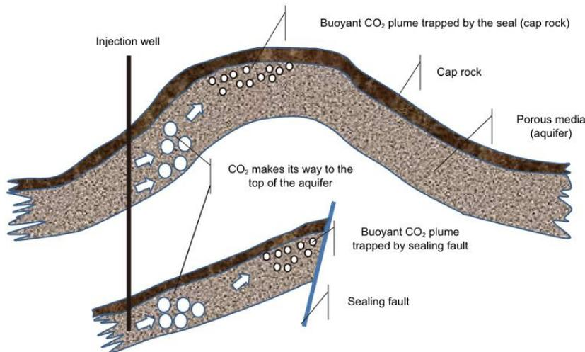
Figure 8 Structural trapping of injected CO<sub>2</sub> as a result of the formation structure. [13]
