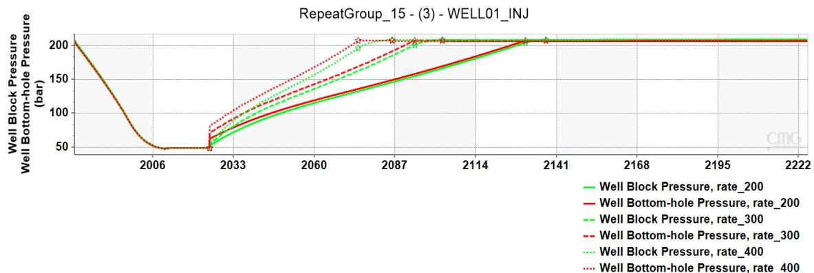
Figure 64 WBHP and Block Pressure profiles
