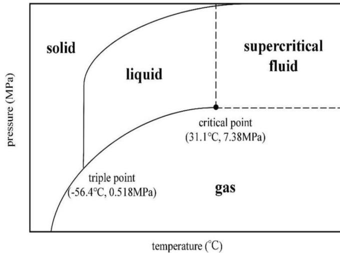
Figure 11 CO<sub>2</sub> phase diagram.
