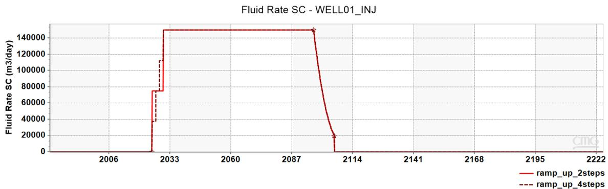
Figure 57 Ramp-Up injection rates: 2 and 4 steps (well 1)
