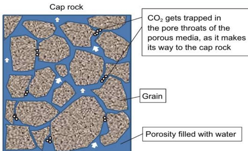
Figure 9 Residual trapping of CO<sub>2</sub> [13]
