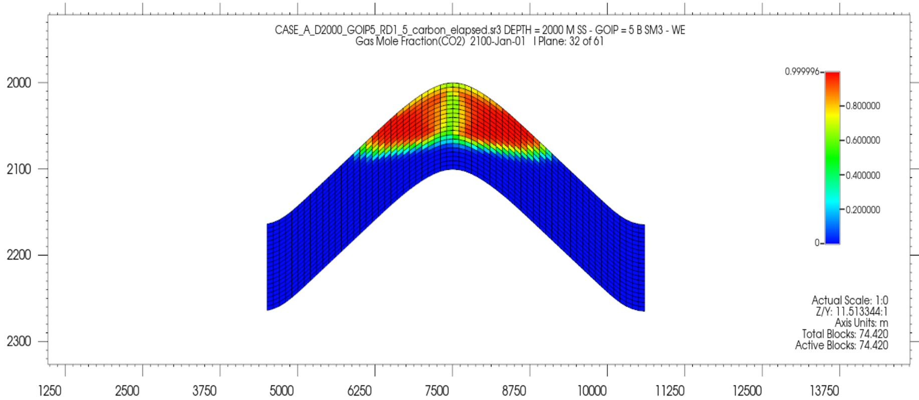
Figure 28 CO<sub>2</sub> injected-case E
