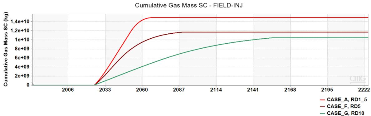
Figure 31 Cumulative CO<sub>2</sub> injected, cases A, F, G
