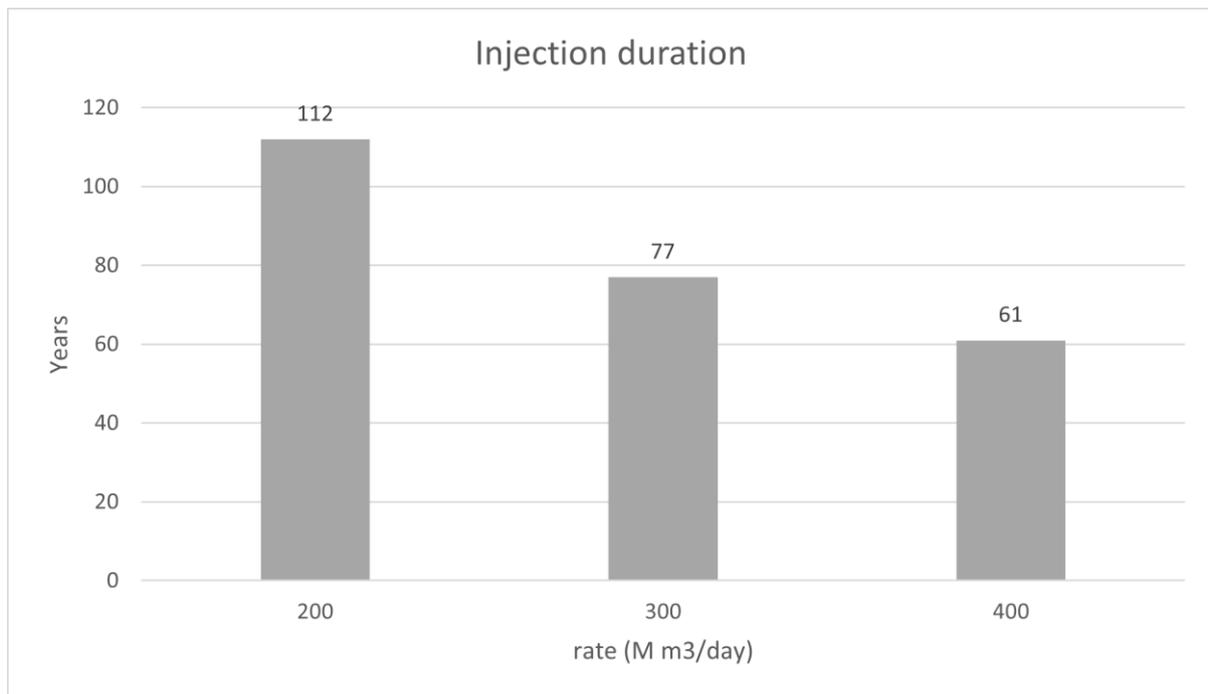
Figure 62 Injection duration for the different constant rates
