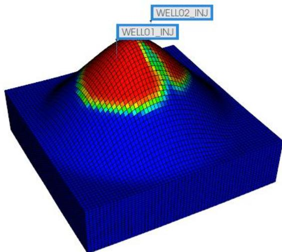
Figure 18 3D representation of model A after CO2 injection
