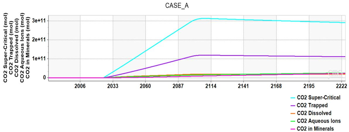
Figure 20 Different trapping mechanisms case A
