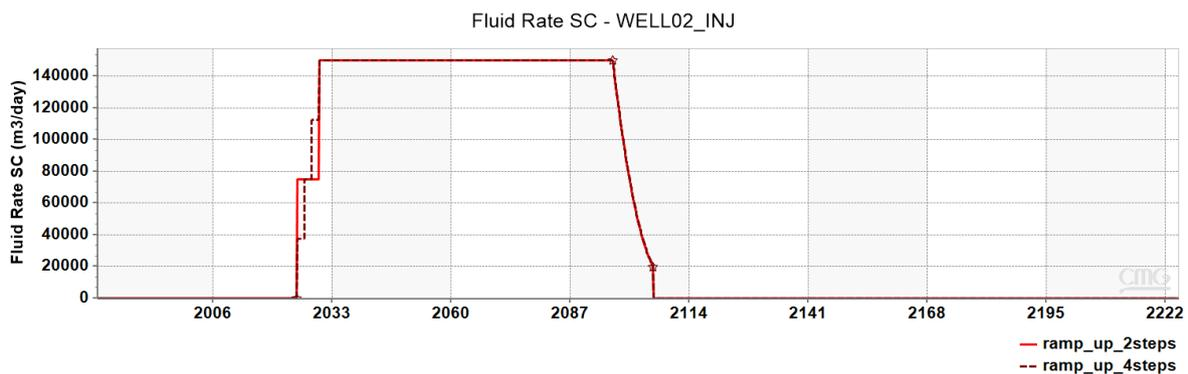
Figure 58 Ramp-Up injection rates: 2 and 4 steps (well 2)
