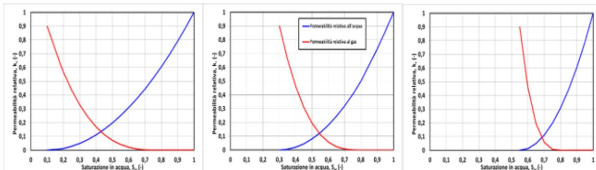
Figure 41 Relative permeability curves according to diff Sw<sub>i</sub>
