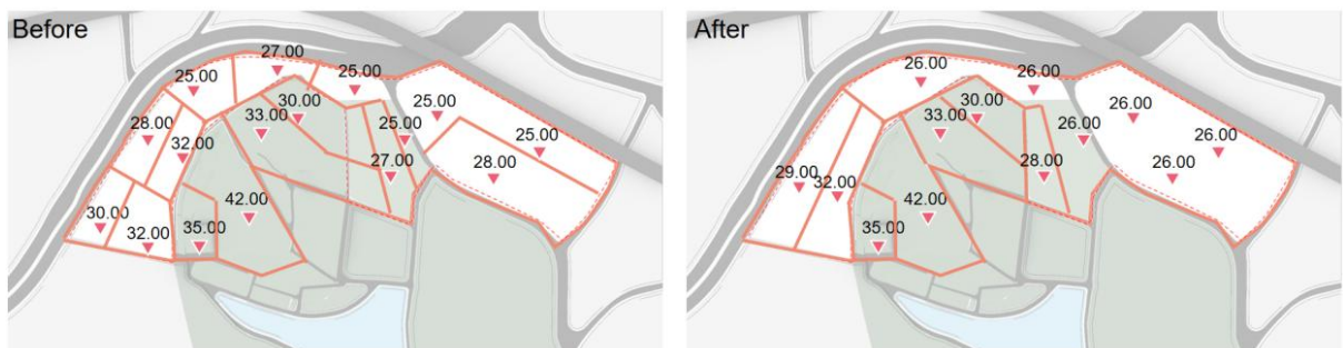
Fig 6-4: Earthwork balance before and after
