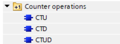
Figure 48 Counter Operation blocks
