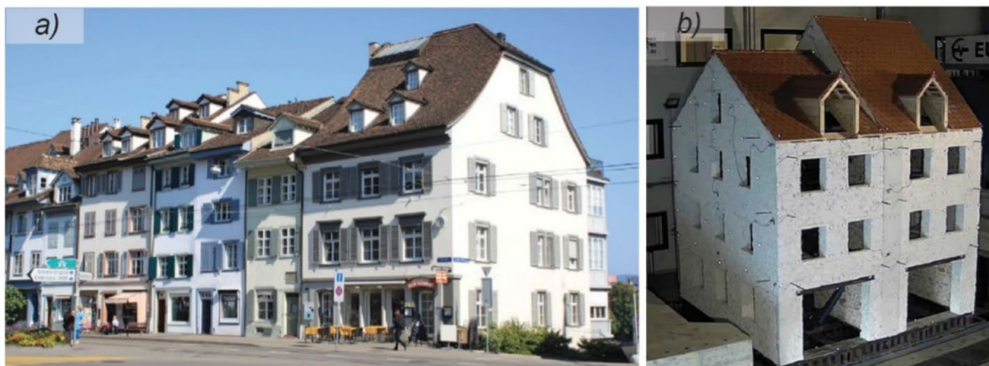
Figure 18: (a) Example aggregate in Basel (Switzerland); (b) Laboratory tested masonry aggregate (8).
