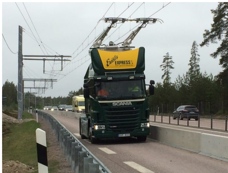
Figure 3: a truck runs with aerial electric feeding on Highway E16, Sweden – from https://shorturl.at/bowCX
